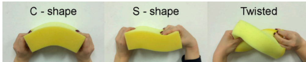
Figure 36: A macroscopic example in which a sponge is deformed by hand, illustrating the relationship between the rotational force and shape. The sponge can be bent in two different ways (left and middle) and twisted (right). Adapted from [178].
