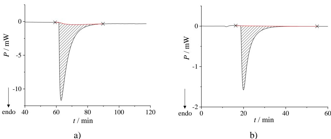
**Slika 55.** Termogrami procesa otapanja a) kokristala benzofenona i difenilamina ( $m = 36,09$  mg) u acetonitrilu ( $V = 1,5$  mL) pri  $25^\circ\text{C}$  proveden u Setaram-Calvetovom kalorimetru i b) metastabilne tekućine benzofenona i difenilamina u molarnom omjeru ( $n(\text{Bzp}) : n(\text{Dpa}) = 1 : 1$ ) ( $m = 21,973$  mg) u acetonitrilu ( $V = 17$  mL) pri  $25^\circ\text{C}$  proveden u TAM IV kalorimetru.
