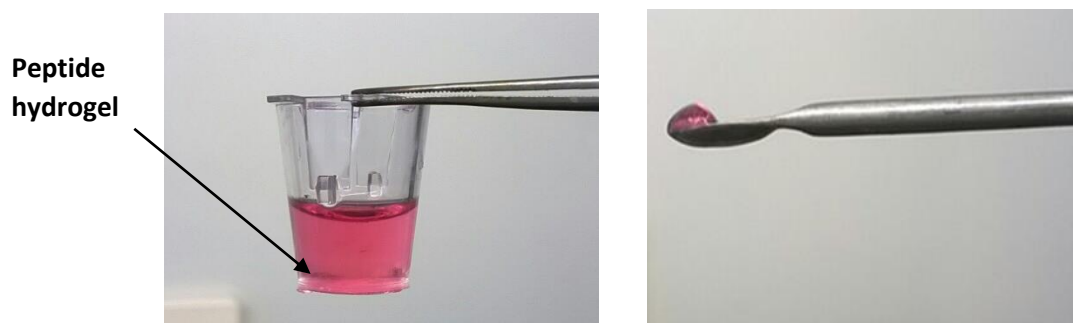
Figure 12. Appearance of cell inserts after 19 days (left). Transparent layer of peptide hydrogel is visible at the bottom of the insert; the rest is chondrogenic medium. Peptide hydrogel taken out of the cell insert (right).
