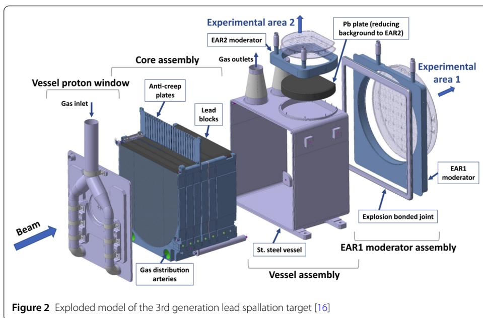
Figure 2 Exploded model of the 3rd generation lead spallation target [16]
