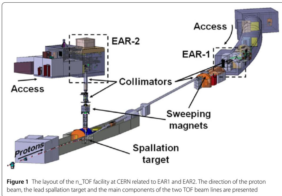
**Figure 1** The layout of the n\_TOF facility at CERN related to EAR1 and EAR2. The direction of the proton beam, the lead spallation target and the main components of the two TOF beam lines are presented
