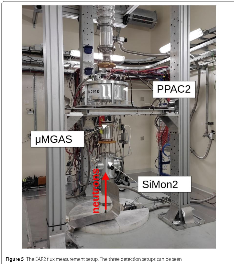
**Figure 5** The EAR2 flux measurement setup. The three detection setups can be seen
