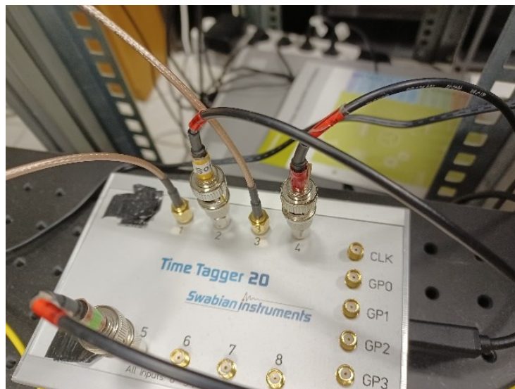
Figure 11. Time tagger module with coaxial cables connected to single photon counting modules (shown in Figure 10). Note that the LEDs are covered with black tape due to influence on the count rate of the detectors. All the sources of light in the laboratory were covered, including from the floor of a slightly elevated laboratory door.
