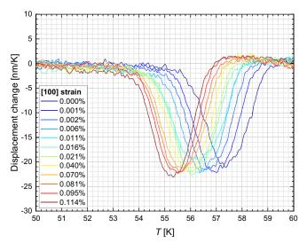
FIG. 11. The anomaly in displacement change  $(\Delta L/\Delta T)$  of the strain cell measured in cooling  $(r=1~{\rm K/min})$  for different applied stresses along the [100] direction. The anomaly temperature coincides with the structural transition temperature  $T_{\rm LTT}=57.5~{\rm K}$  at zero applied stress. For increased strain values shown in the legend, the anomaly shifts to a lower temperature of 55.5 K.
