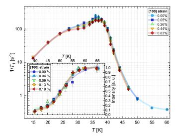
FIG. 3. Temperature dependence of  $^{139}T_1^{-1}$  measured with stress applied along [100] and  $H \parallel$  [001]. Lines are guides to the eyes. The inset shows the NQR measurements of copper B-line at  $\sigma_{[100]}$ . Lines are fits to the phenomenological function I(T) (see the text). The legend shows the values of induced strain.
