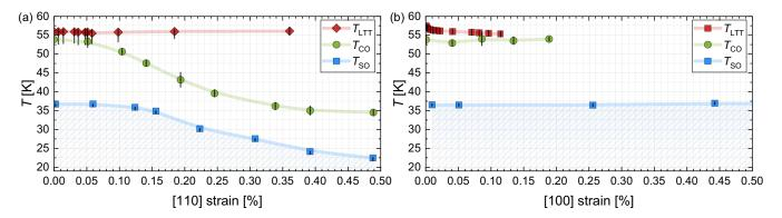
FIG. 4. Strain-temperature phase diagram for  $H \parallel c$  and stress applied (a) along the [110] direction, and (b) along the [100] direction. The data points are extracted from the data of Figs. 2 and 3 and show that  $\sigma_{[110]}$  reduces  $T_{SO}$  (blue) and  $T_{CO}$  (green), even though the onset of LTT structural phase remains the same (red). However,  $\sigma_{[100]}$  does not change  $T_{SO}$  at all, while  $T_{LTT}$  shows a mild drop. Lines are guides to the eyes.
