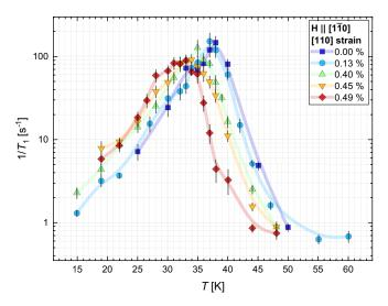
FIG. 5. Temperature dependence of  $^{139}T_1^{-1}$  measured with stress  $\sigma_{[110]}$  and  $H \parallel [1\overline{1}0]$ . Lines are guides to the eyes. The suppression of  $T_{\rm SO}$  is greatly reduced. The legend shows the values of measured strain.
