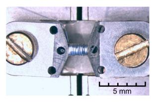
FIG. 7. NMR coil with the sample in the uniaxial cell.
