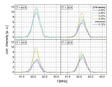
FIG. 8.  $^{139}$ La NMR spectra (central transition) under different [110] uniaxial strains, at chosen temperatures above and below  $T_{SO}$ .
