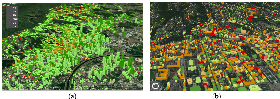
Figure 2. Damage to residential and commercial–residential buildings on: (a) a perspective view of the city of Zagreb according to usability tags (colors) and gross floor areas of buildings (heights of columns) and (b) a perspective view of the historical center according to buildings’ usability tags from the GIS-based Building Usability Database (source: Croatian Centre for Earthquake Engineering—CCEE).
