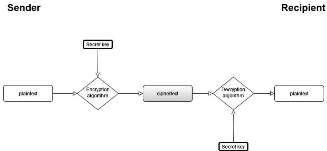
Figure 2.1: Symmetric encryption
