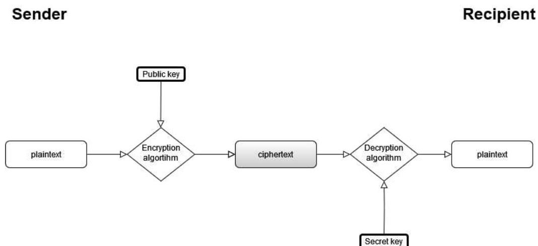
Figure 2.2: Asymmetric encryption
