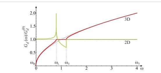
**Figure 2.** The density of electron states (DOS) of a reconstructed system described by the bands equation (2.7) as a function of the scaled energy  $\omega$  in units of  $G_d^{(0)}$  for  $\eta=0.2$ . Full green and red lines represent the 2D and 3D case respectively. The dashed lines represent the 2D and 3D free electron DOS equation (3.8).
