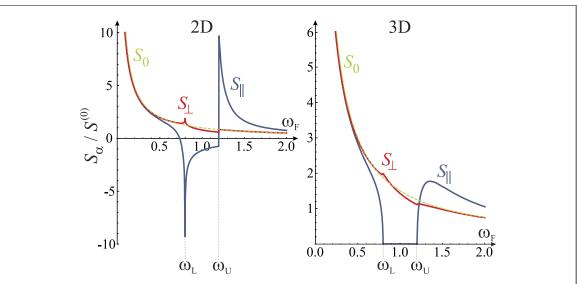
**Figure 4.** Direction-dependent Seebeck coefficient,  $S_{\parallel}$  and  $S_{\perp}$ , as a function of scaled Fermi energy  $\omega_F$  for the 2D and 3D system described by equation (2.7) in units of  $S_d^{(0)}$  for  $\eta=0.2$  and  $m=m_{\rm e}$ . The free electron gas value  $S_0$  equation (4.8) is presented by the green dashed line.
