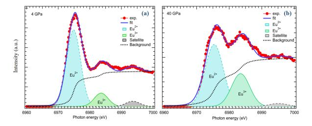
Figure 3.6: Examples of the fitting Eu  $L_3$  HERFD XAS spectra at 4 GPa (a) and 40 GPa (b) to extract Eu<sup>2+</sup> and Eu<sup>3+</sup> components.
