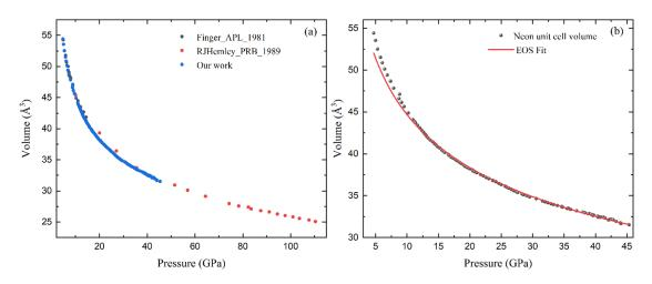
Figure C.2: (a) Pressure dependent unit cell volume of neon obtained from XRD experiment compared with data in Ref. [94] and [98]. (b) Pressure dependent unit cell volume of neon and the result of  $3^{rd}$  order BM EOS fitting with  $V_0 = 88.967 \text{ Å}^3$  [98].
