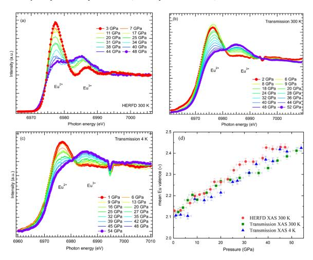
Figure 3.7: The Eu  $L_3$  XAS spectra of powder EuIrGe<sub>3</sub> as function of pressure. (a) HERFD XAS at 300 K, spectras are normalized on higher energy end after substracting constant background below the edge. (b) Transmission XAS at 300 K, a glitch due to optics is visible at 6995 eV, (c) Transmission XAS at 4 K. (d) The mean Eu valence as function of pressure obtained from all three experiments.
