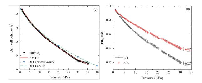
Figure 3.17: (a) EuRhGe<sub>3</sub> unit cell volume as function of pressure with  $3^{rd}$  order BM EOS Fit. DFT calculated unit valume and EOS Fit is also presented. (b) Normalized a, c lattice parameters of EuRhGe<sub>3</sub> as a function of pressure.
