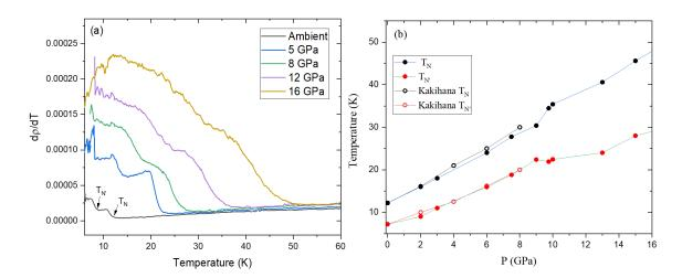
Figure 3.25: (a): First order derivative of resistivity curve of EuIrGe<sub>3</sub> (Exp. 3) at different pressures. Magnetic ordering temperature  $T_N$  and  $T_{N'}$  are extracted from resistivity derivative, presented by arrows at ambient pressure curve. (b): Pressure evolution of magnetic ordering temperatures  $T_N$  and  $T_{N'}$  of EuIrGe<sub>3</sub> compared with the reported values in Ref. [44].
