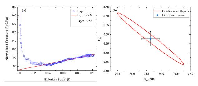
Figure C.3: Visual quality assessment of EOS fitting. (a) Normalized pressure F vs Eulerian strain f plot of EuCoGe<sub>3</sub>. The red line presents the linear fit by using  $F = B_0 + [3B_0 (B'_0 - 4)f]/2$ . (b) The confidence ellipse between  $B_0$  and  $B'_0$ . Confidence ellipse is presented for 99.73 percent confidence level.
