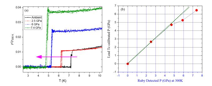
Figure 2.4: (a): Normalized electric resistivity curves of lead at selected pressure. Effect of increase in pressure on  $T_c$  of lead can be seen as a shift towards low temperatures. (b): The obtained pressures from lead  $T_c$  and the pressure determined by ruby fluorescence at 300K. These experiments were performed at the institute of physics, Zagreb.
