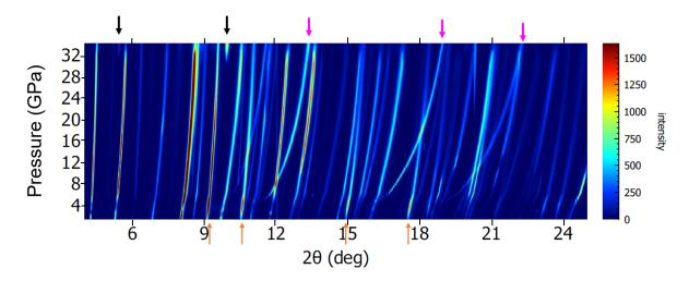
Figure 3.19: Contour map of synchrotron X-ray diffraction intensities in the pressure range of 0.5–34 GPa. The pressure evolution of Bragg peak positions contains EuIrGe<sub>3</sub> (main phase), gold (standard material), neon (pressure-transmitting medium), and rhenium (gasket). The black arrows (top) represent rhenium, which appears around 30 GPa. The magenta arrow (top) represents neon as the pressure-transmitting medium, and the yellow arrows (bottom) represent gold Bragg peaks.
