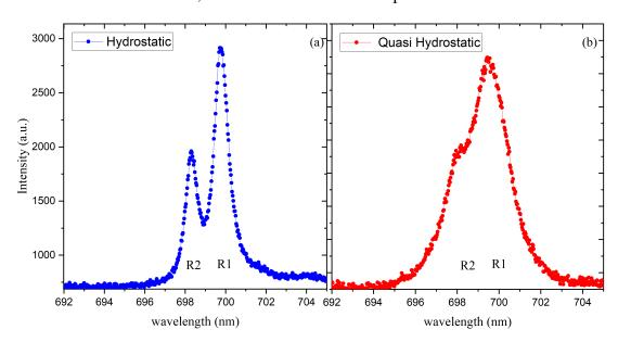
Figure A.1: Ruby fluorescence spectra at 14 GPa. (a) hydrostatic pressure. (b) quasi or non-hydrostatic pressure.
