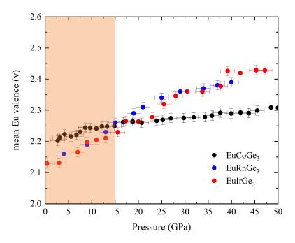
Figure 4.1: Mean Eu valence as function of pressure of EuCoGe<sub>3</sub>, EuRhGe<sub>3</sub> and EuIrGe<sub>3</sub>. Shaded region is showing the coexisting intermediate valence and antiferromagnetism.
