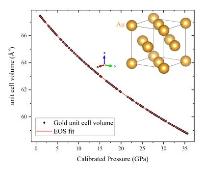
Figure 2.3: Unit cell volume of gold and EOS fitting as a function of calibrated pressure. Inset shows the crystal structure of gold (Fm-3m, 225) drawn by VESTA [26]. These experiments were performed at the Soleil synchrotron, France.
