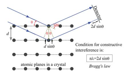
Figure 2.13: Schematic representation of Bragg's law conditions.
