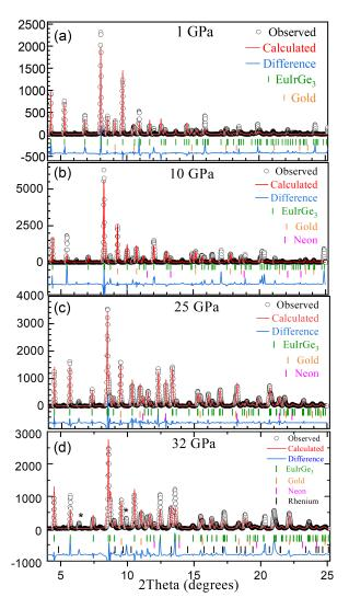
Figure 3.20: Integrated synchrotron XRD patterns of EuIrGe<sub>3</sub> with the results of Rietveld refinement at (a) 1 GPa, (b) 10 GPa, (c) 25 GPa, and (d) 32 GPa. The vertical bars indicate Bragg peak positions of EuIrGe<sub>3</sub> (green), gold (orange), neon (magenta) and rhenium (black). Some unindexed peaks are also visible in diffractogram shown with \*.
