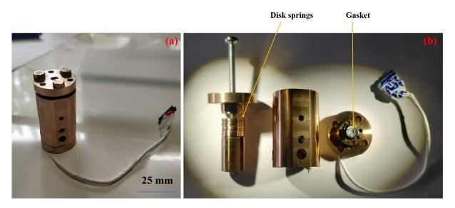
Figure 2.5: The BeCu DAC for electric resistivity measurements under pressure. (a): Assambled DAC. (b): Different components of the DAC, disk springs, piston, gasket, and diamond anvils.
