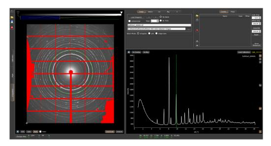
Figure C.5: Dioptas windows of raw XRD (left) and extracted diffractogram (right) with mask. Application of mask removes the peaks generated from diamonds and/or detector.
