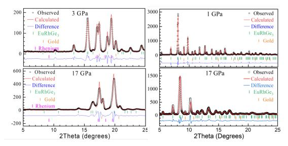
Figure C.1: Comparison of laboratory and synchrotron XRD data of EuRhGe3 at low and high pressures.
