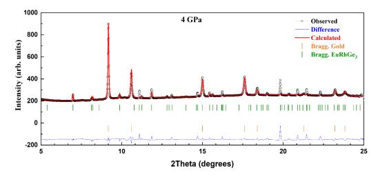
Figure C.6: Synchrotron powder XRD pattern of EuRhGe<sub>3</sub> along with the results of Rietveld refinement with neon PTM, showing the dominance of gold signal over EuRhGe<sub>3</sub>.
