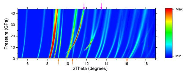
Figure 3.12: Contour map of synchrotron x-ray diffraction intensities collected in the pressure range 1–45 GPa, for EuCoGe<sub>3</sub> (main phase), gold (standard material), and neon (pressure medium). The magenta arrows (top) and the yellow arrows (bottom) of the contour map represent the main peak positions of neon and gold respectively.
