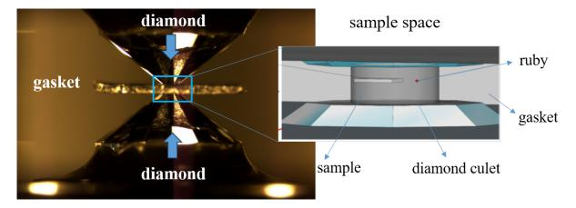
Figure 2.1: Side view of a diamond anvil cell. Two opposing diamonds attached on backing plates, and a gasket is pressed in between diamond culets. A magnified view of sample space with pressure indicator ruby in it.
