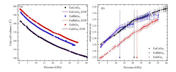
Figure 4.2: (a) Unit cell volume as function of pressure for all three compounds with respective EOS fitting. (b) The axial ratio (c/a) for EuTGe<sub>3</sub>, showing the kink at 21 GPa, 13 GPa and 22 GPa in EuCoGe<sub>3</sub>, EuRhGe<sub>3</sub> and EuIrGe<sub>3</sub> respectively. The linear fit are presented for EuRhGe<sub>3</sub>.
