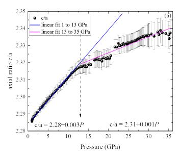
Figure 3.18: Pressure dependence of the axial ratio (c/a) of EuRhGe<sub>3</sub>. Straight lines emphasize linear behavior. To emphasize the change of slope, the linear fit of the low perssure region is extended into the high pressure region.
