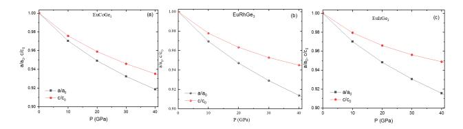
Figure B.2: Relative pressure variation of the DFT calculated lattice parameters of (a) EuCoGe<sub>3</sub>, (b) EuRhGe<sub>3</sub>, and (c) EuIrGe<sub>3</sub>.
