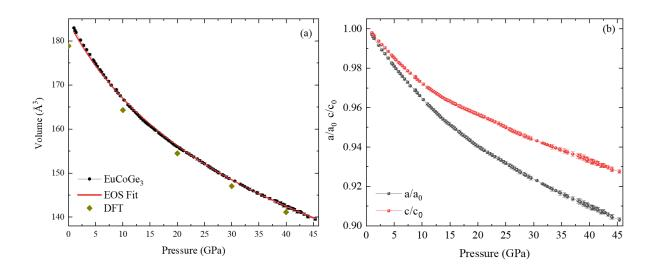
Figure 3.14: (a) XRD and DFT calculated unit cell volume of EuCoGe<sub>3</sub> as a function of pressure and the result of  $3^{rd}$  order BM EOS Fit. (b) Normalized a, c lattice parameters of EuCoGe<sub>3</sub> as a function of pressure. The  $a_0$  and  $c_0$  values correspond to the obtained lattice parameters of the lowest pressure.
