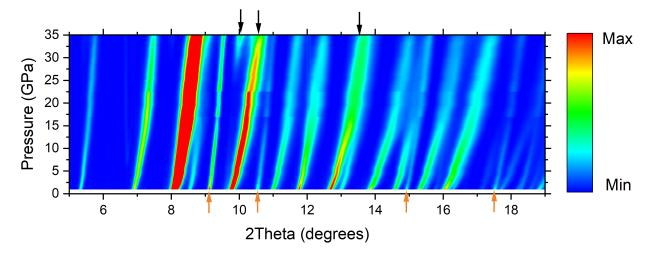
Figure 3.16: Contour map of synchrotron x-ray diffraction intensities in the pressure range from 1 to 35 GPa. The pressure evolution of Bragg peak positions contains EuRhGe<sub>3</sub> (main phase), gold (standard material), and rhenium (gasket) which appears above 25 GPa. The black arrows (top) and yellow arrows (bottom) of the contour map represent the main peak positions of rhenium and gold respectively.
