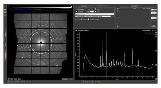
Figure C.4: Dioptas windows of raw XRD image (left) and extracted diffractogram (right) without mask.
