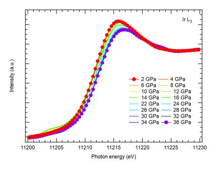
Figure 3.10: Pressure dependent Ir  $L_3$  edge XAS spectra of EuIrGe<sub>3</sub> in transmission mode at 300 K.
