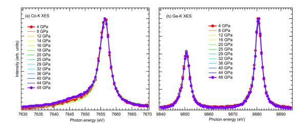
Figure 3.4: (a) Co  $K_{\beta}$  and (b) Ge  $K_{\alpha}$  emission spectra of EuCoGe<sub>3</sub> as function of pressure.
