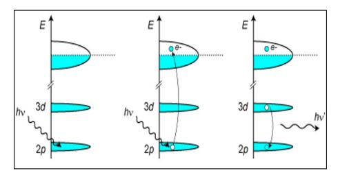
Figure 2.10: Schematic of Eu  $L_3$  HERFD XAS - High energy photon is exciting core electron to the unoccupied states. Then one electron from 3d level relaxes into the 2p core hole emitting photon with energy of hv'. This fluorescence signal is detected in HERFD XAS.
