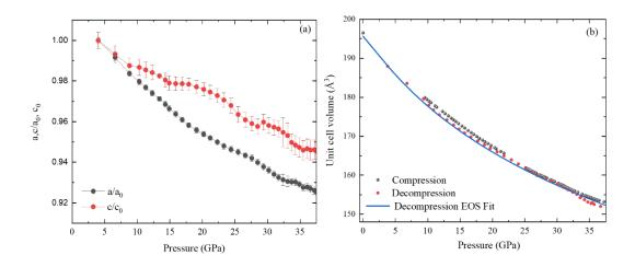
Figure C.7: (a) Pressure variation of the lattice parameters of EuRhGe<sub>3</sub>. (b) Pressure-dependent unit cell volume of EuRhGe<sub>3</sub> by using neon PTM. Black and red dots represent the data obtained during compression and decompression processes, respectively. Here, the EOS fit is applied to the decompression data.
