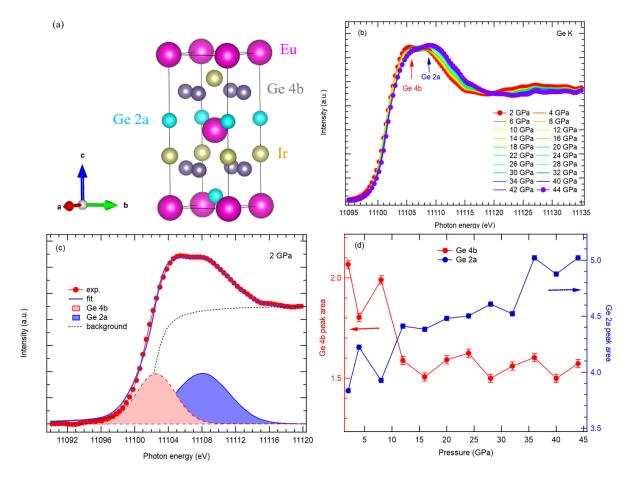
Figure 3.9: (a) Unit cell of EuIrGe<sub>3</sub>. Ge ions occupy the 2a and 4b Wyckoff positions. (b) Pressure dependent Ge *K* XAS of EuIrGe<sub>3</sub> in transmission mode at 300 K. (c) Spectra fitting of Ge *K* XAS and (d) spectral areas of the Ge 4b to Ge 2a peaks as a function of pressure.
