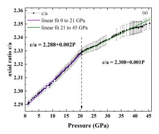
Figure 3.15: The axial ratio of EuCoGe<sub>3</sub> as function of pressure. The change of the slope was observed around 21 GPa indicated with an arrow.
