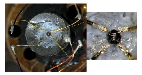
Figure 2.9: **Left**: Sample connections for electric resistivity measurement under pressure by four probe method. The outer wires are made of the gold with 50  $\mu$ m thickness. **Right**: The magnified view of the sample space.
