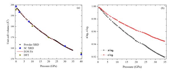
Figure 3.21: (a) Powder XRD, Single crystal XRD and DFT calculated unit cell volume of EuIrGe<sub>3</sub> as function of pressure.  $3^{rd}$  order BM EOS fitting for powder XRD data is also provided. (b) Anisotropy along a and c- axis as function of pressure.
