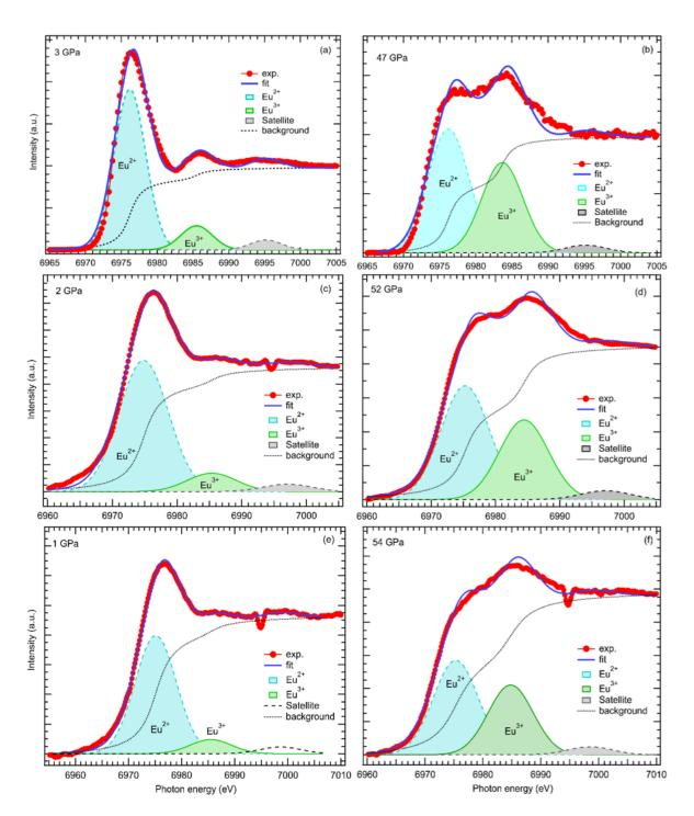
Figure 3.8: The fittings of the Eu  $L_3$  XAS spectra of EuIrGe<sub>3</sub> at selected pressures in (a, b) HERFD XAS at 300 K, (c, d) Transmission XAS at 300 K, and (e, f) Transmission XAS at 4 K.
