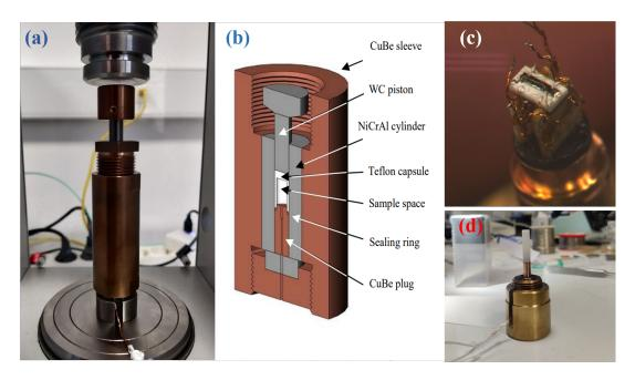
Figure B.3: (a) Assembled Piston cylinder cell in hydraulic press. (b) Illustration of the cross section of a piston-cylinder-type NiCrAl pressure cell, Taken from [97]. (c) Sample connected with the outer connections, sample is glued to ceramic bases. (d) Samples are loaded inside a 20 mm long and 5 mm diameter teflon tube.
