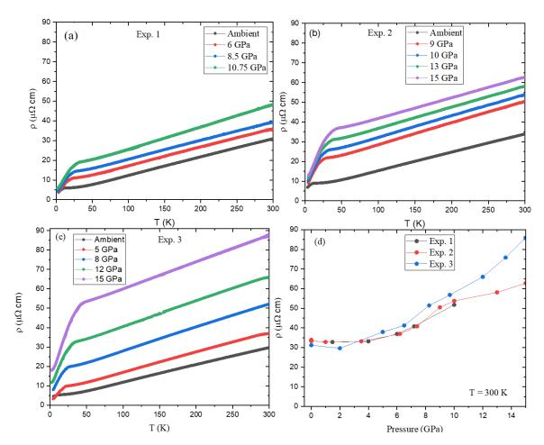
Figure 3.24: Temperature dependent electric resistivity of EuIrGe<sub>3</sub> under pressure. (a): Exp. 1 (b): Exp. 2, (c): Exp. 3, and (d): Resistivity at 300 K of three samples as function of pressure.
