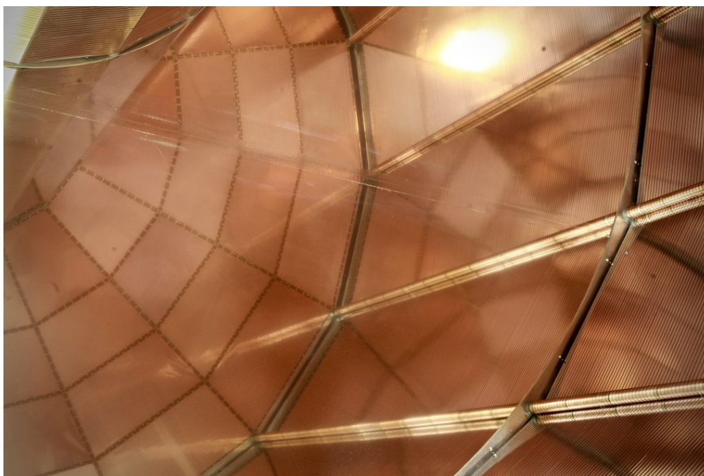
Figure 47. An image inside the TPC. The central electrode reflects a view of the field cage and the readout chambers. The subdivision of each sector into four GEM stacks can be seen.
