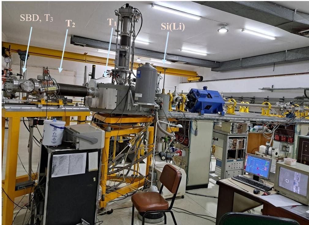
**Figure 3.2.** Side view of the *Total IBA chamber at iThemba LABS TAMS*
