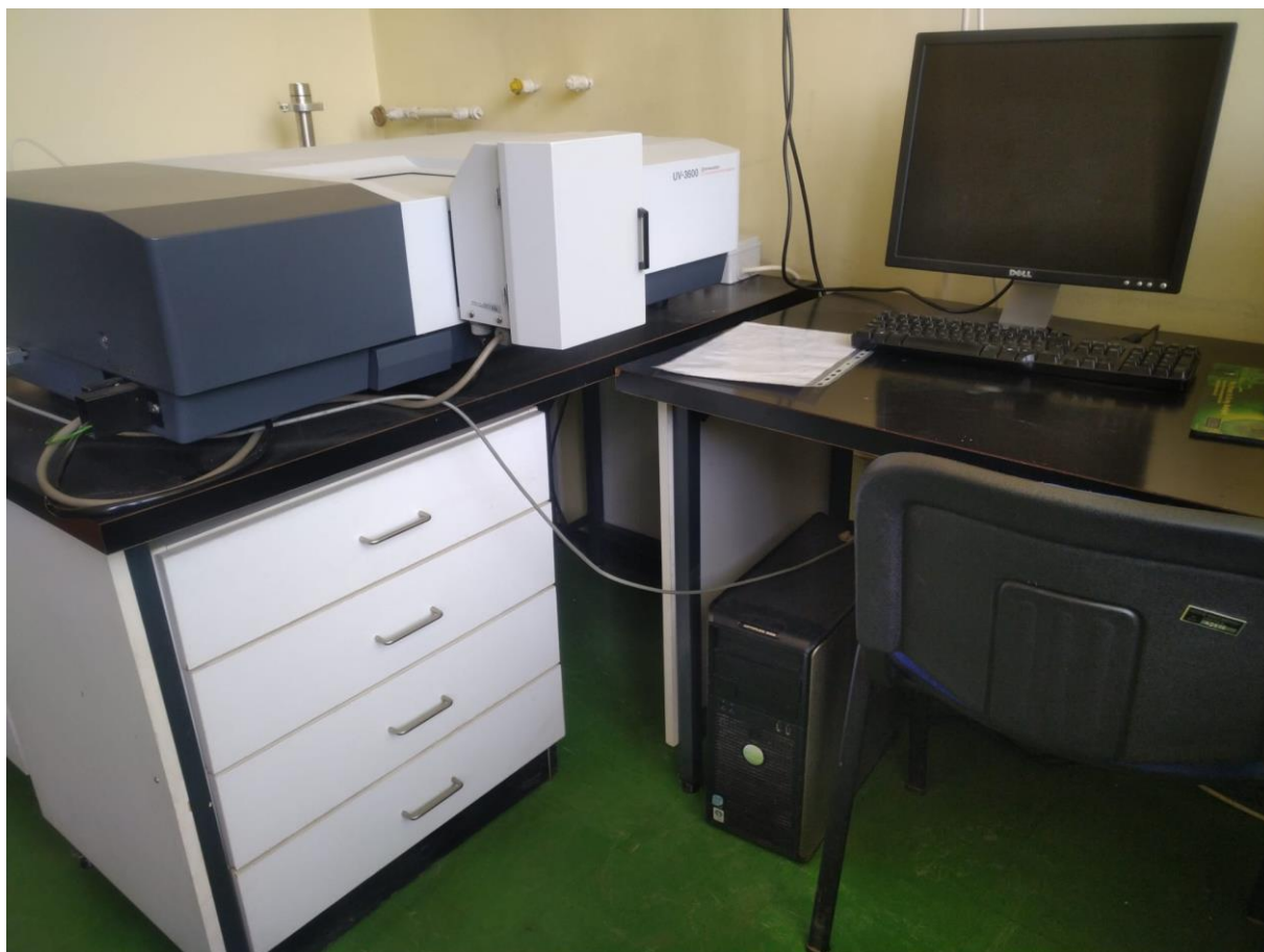
Figure 6.7 UV-3600 Shimadzu UV-Vis-NIR spectrometer from the Division of Materials Chemistry at Ruđer Bošković Institute
