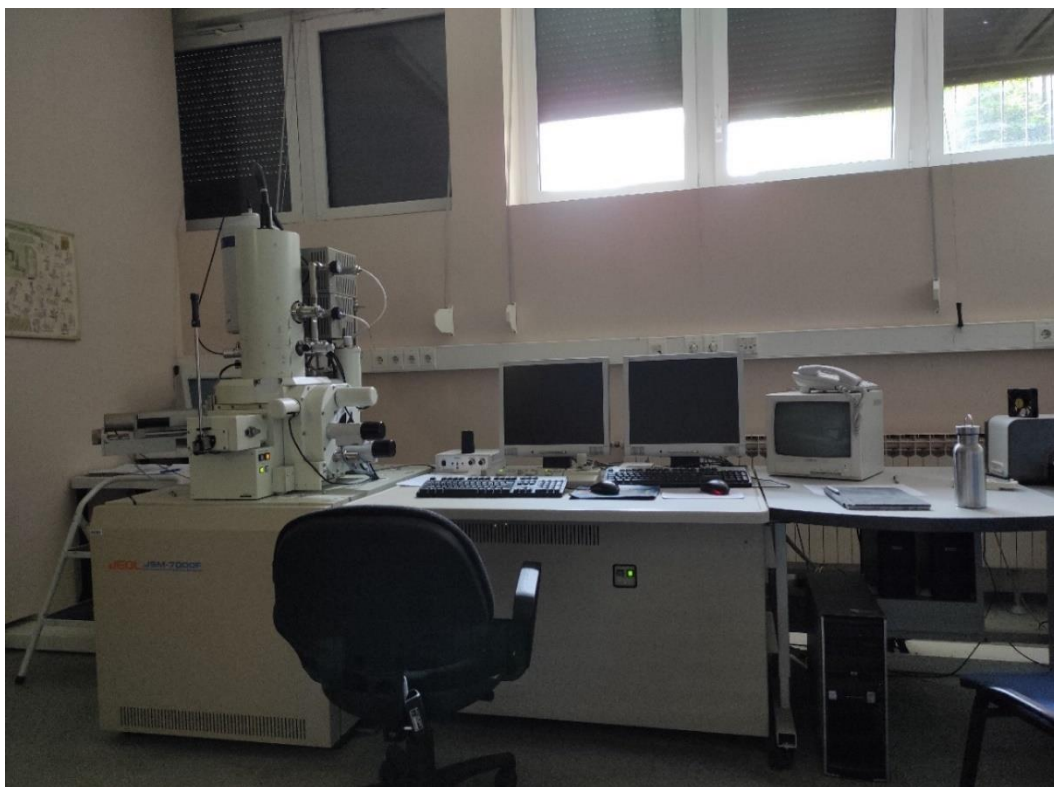
Figure 6.8 JEOL JSM-7000 scanning electron microscope together with energy-dispersive X-ray spectroscopy device from the Division of the Materials Chemistry at Ruđer Bošković Institute
