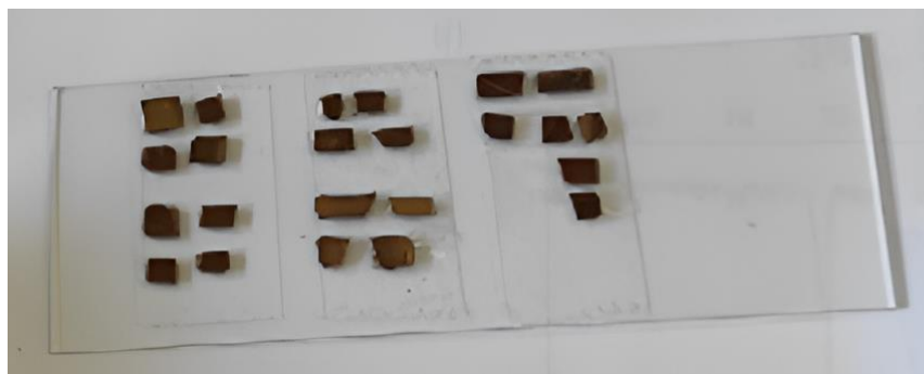
Figure 6.11 Photograph of SERS substrates prepared for Raman measurements
