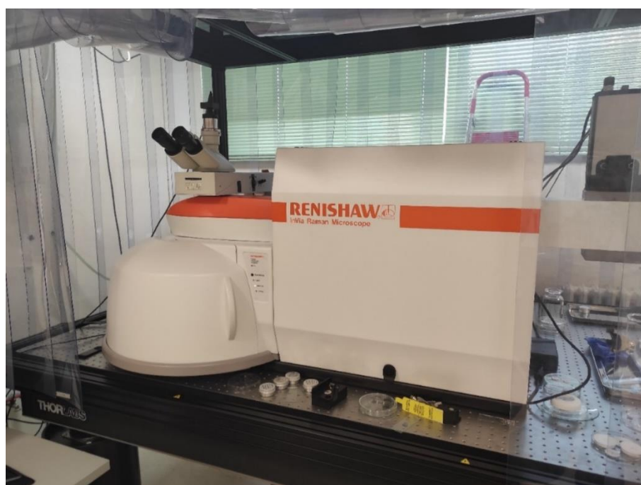
Figure 6.10 inVia™ Raman microscope from the Division of Materials Physics, Ruđer Bošković Institute
