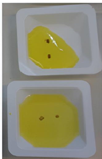
Figure 6.6 Photograph of pSi and pSi PhC samples during the synthesis of gold nanoparticles
