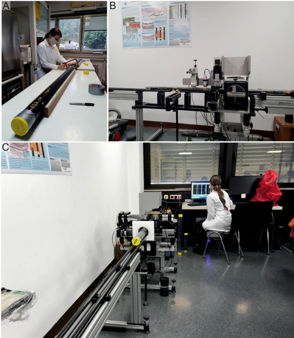
Figure 4.6 A. Cutting the sediment cores into 1.4 m long segments. B. Geotek Multi-Sensor Core Logger. C. Analysis of PROK sediment cores with a core logger.
