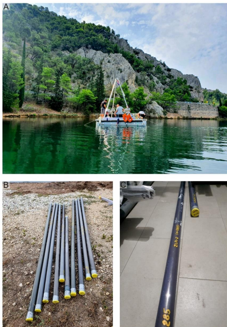
Figure 4.3 Sediment coring. A. Floating research coring platform „Q2“. B. Sediment cores PROK collected in the Krka River estuary. C. Sediment cores ZLA collected in the area of the submerged Pleistocene delta.
