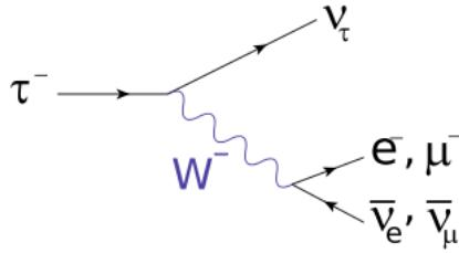
**Figure 5.23:** Feynman diagram of a leptonic  $\tau$  decay
