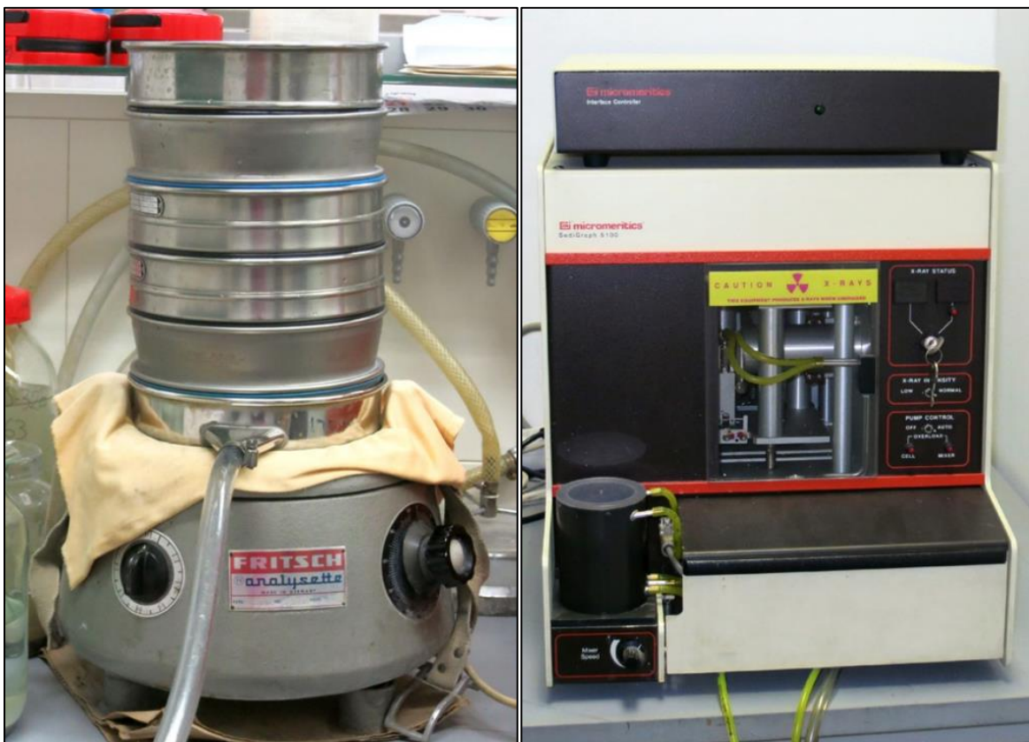
Figure 4.6. Wet sieving and sedigraph method for determining grain size in sediment (Division for Geology and Paleontology, Department of Geology, Faculty of Science, Zagreb).
