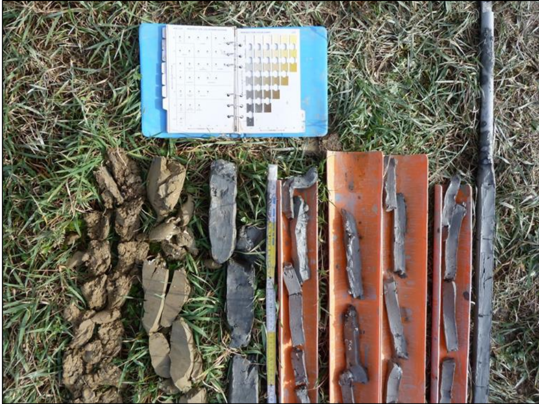
Figure 4.4. Description of the extracted cores on the field with color chart.
