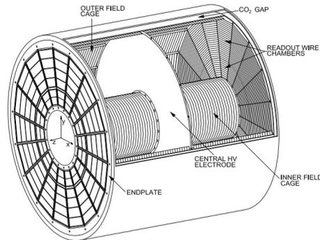
Fig. 4.5 Schematic of the TPC field cage [51].
