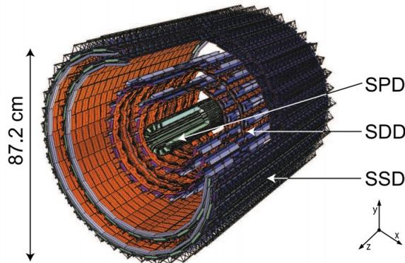
Fig. 4.4 Schematic of the ALICE Inner Tracking System [50].
