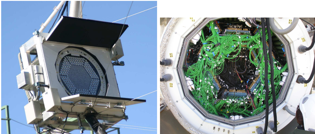
Figure 2.5 Front and back view of the old MAGIC-I camera, with pixels of two different sizes.
