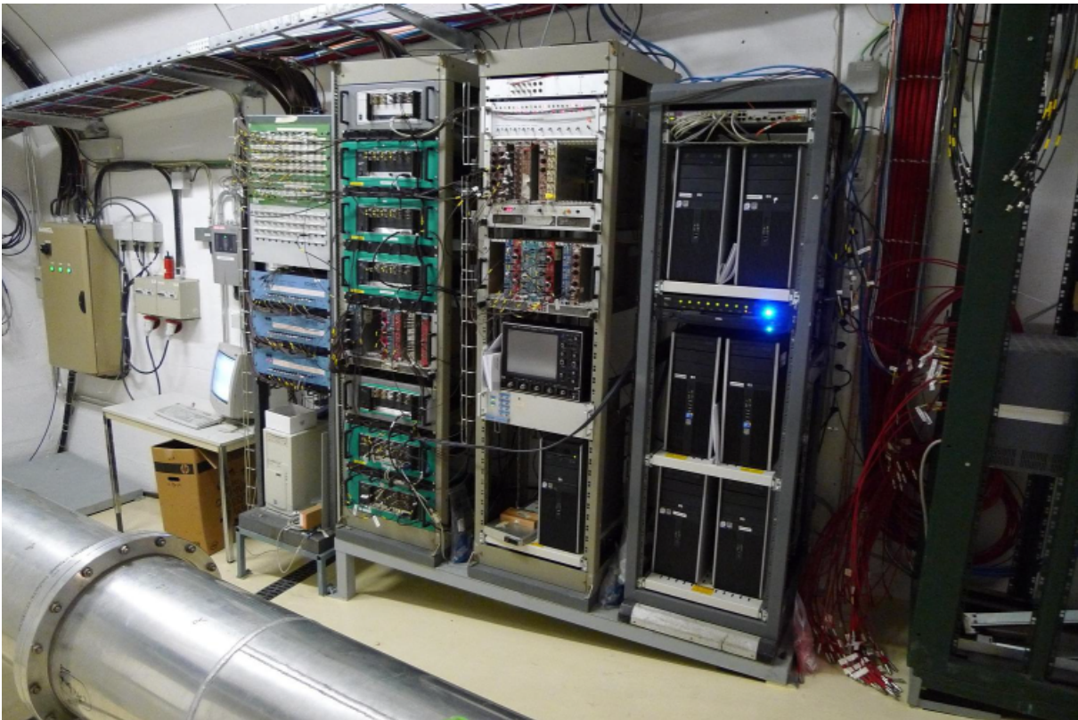
Figure 2.9 — Digital data acquisition system at n_TOF.
