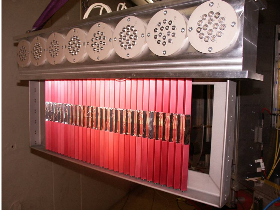
Figure 3.5: The HI detector array seen from the exit of the dipole magnet. CsI(Tl) crystals are wrapped by aluminum foils. The PMTs and bases are in the red housing. Above the detectors there are vacuum-tight connectors for a signal readout and a high voltage supply.
