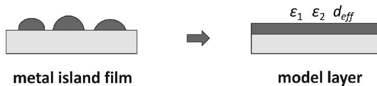
Figure 2.7 MIF is modelled with a homogeneous layer with effective dielectric function and layer thickness.
