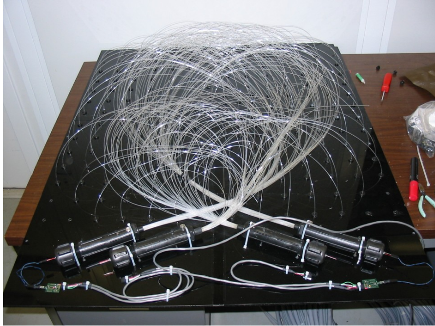
Figure 3.13: The LED panel used to monitor the cell stability. The panel was installed in front of the face of each detector, providing light pulses that would allow monitoring cell stability. One can see the two driver modules and four fiber bunches.
