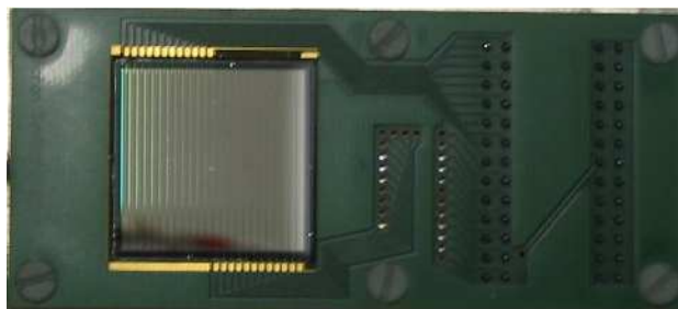
Figure A.1: Double-sided silicon strip detector BB2. Manufactured by Micron Semiconductors Ltd.
