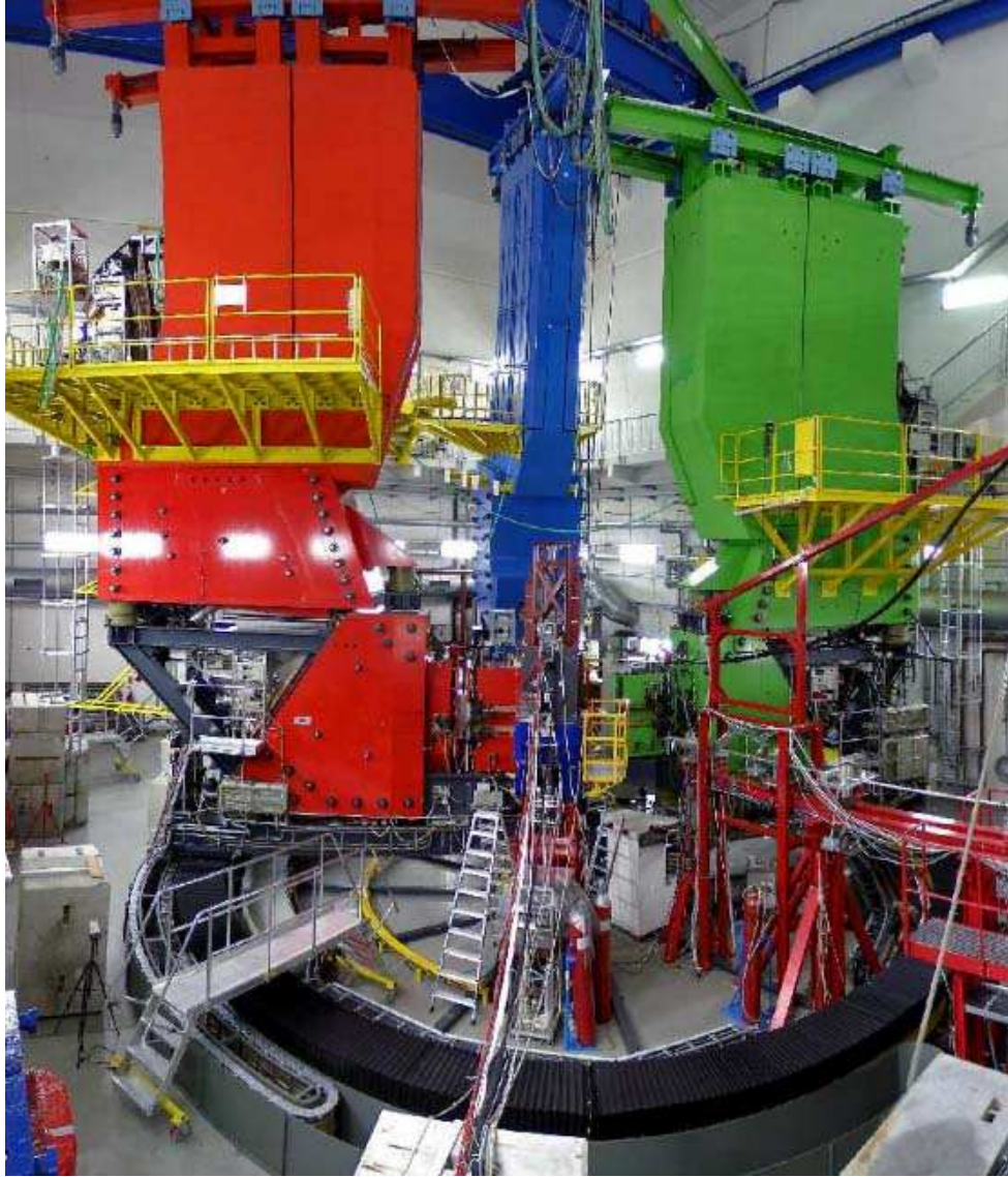
Figure 2.2: The A1-hall with the 3 magnetic spectrometers. From left to right the spectrometers are labeled as A (red), B (blue) and C (green). The electron beam is coming through the pipe from the left side.
