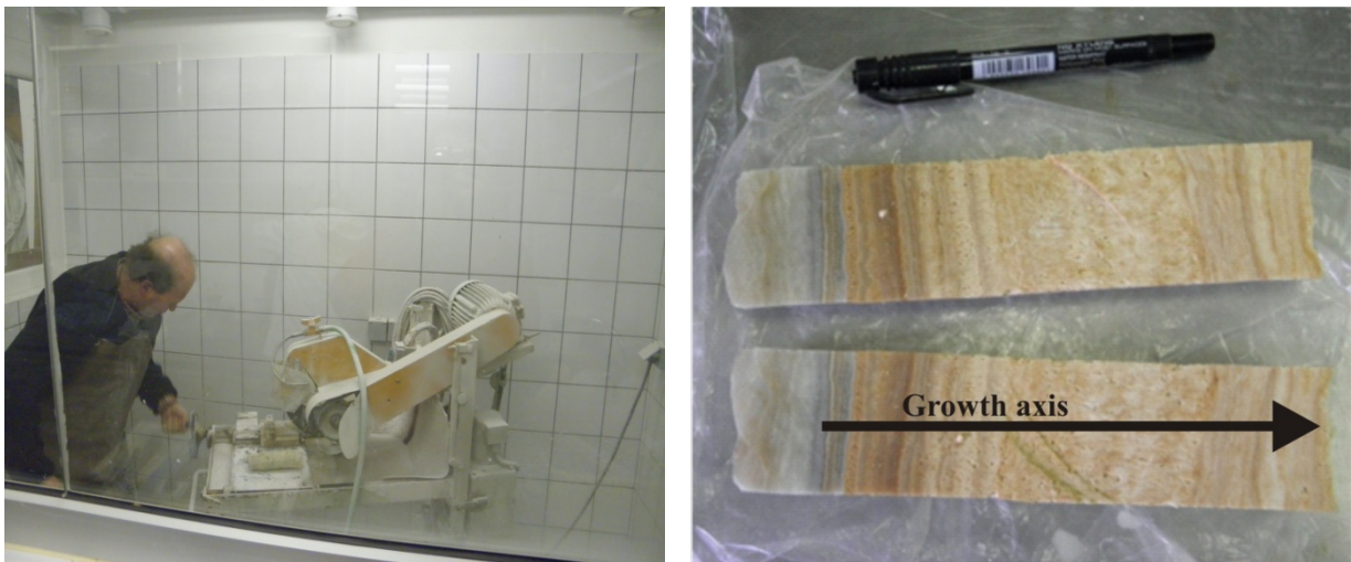
Figure 5.17 Diamond saw for cutting the speleothems (left), and both halves of a core drilled from an old stalagmite (right).
