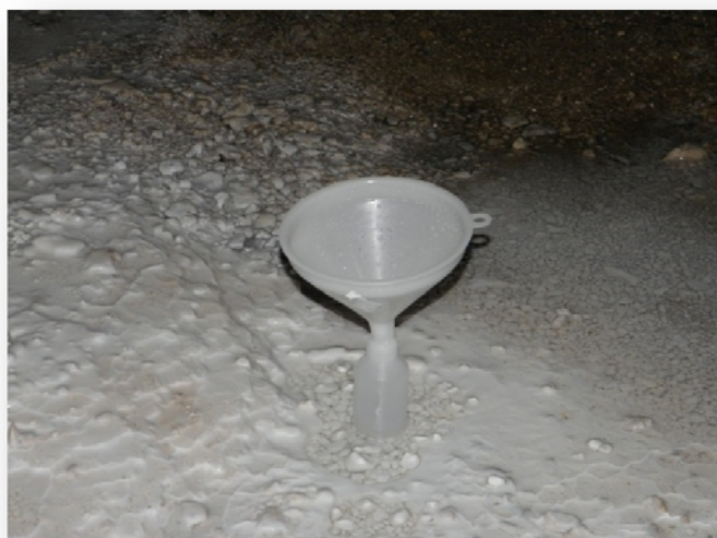
Figure B.4 Collection of drip water in narrow neck HDPE bottle
