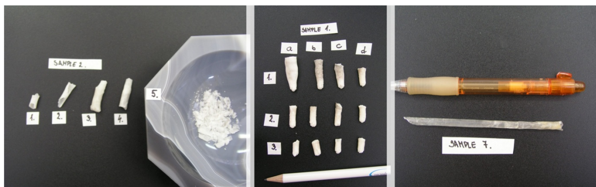
Figure 5.10 Recent carbonate samples and agate mortar for homogenization of a samples.
