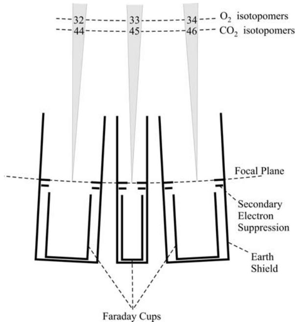
Figure 2.15 Faraday cups settings in IR mass spectrometer Delta<sup>plus</sup> XP (Thermo Scientific)
