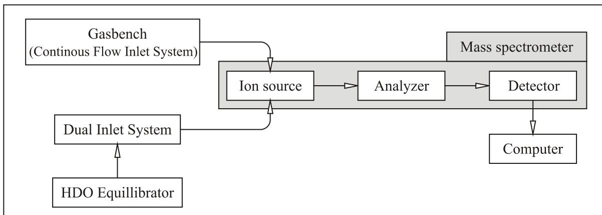
Figure 2.7 Schematic view of an experimental setup of a mass spectrometer with periphery units
