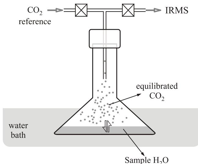
Figure 5.19 Schematic view of equilibration procedure in the HDO equilibration unit.
