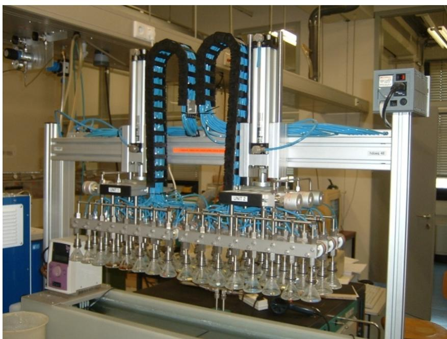
Figure 5.18 Set of 48 bottles prepared for water equilibration in water bath at constant temperature.
