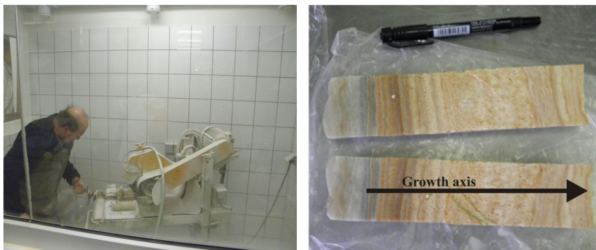
Figure 5.17 Diamond saw for cutting the speleothems (left), and both halves of a core drilled from an old stalagmite (right).
