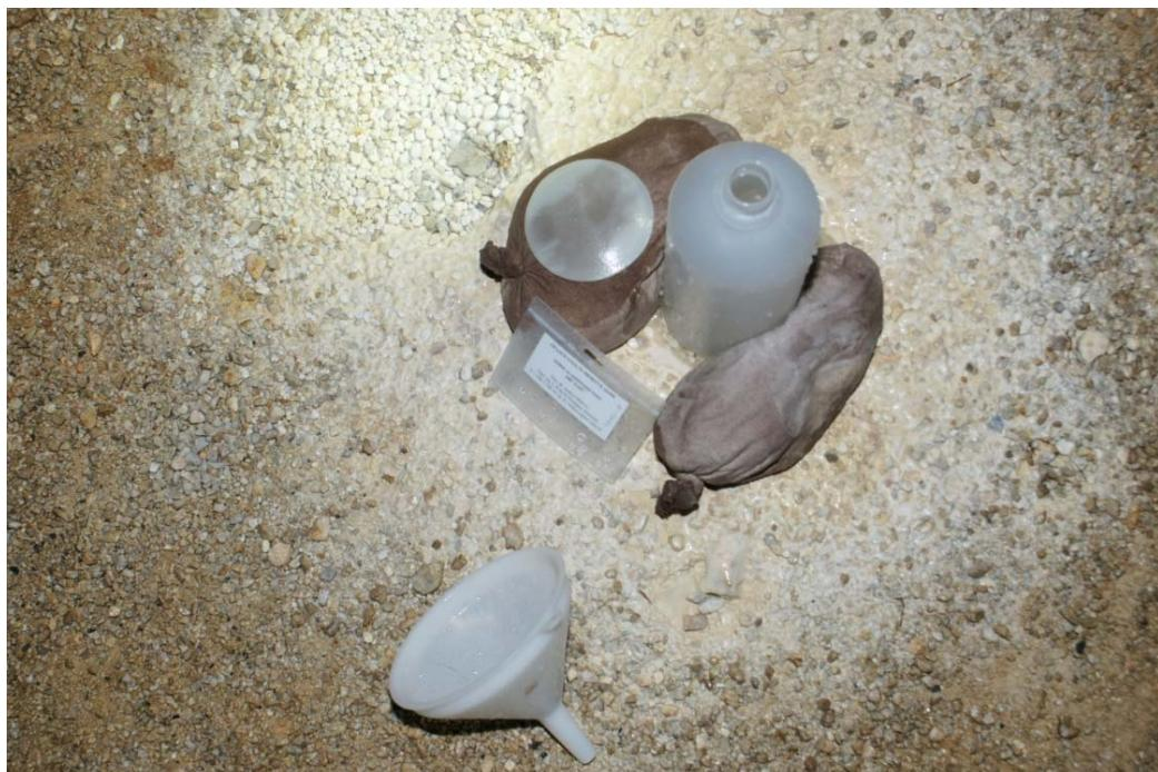
Figure 5.12 A watch glass plate on a sampling site.
