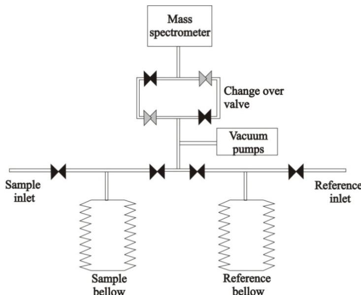
Figure 2.8 Schematic representation of Dual inlet system
