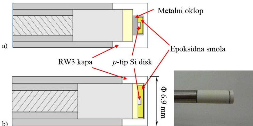
Slika 2.13 Cilindrični poluvodički silicijski detektori *p*-tipa: a) Diode P PTW60016 i b) Diode E PTW60017. (Izvor: Cranmer-Sargison G, Weston S, Evans J A, et al. Monte Carlo modelling of diode detectors for small field MV photon dosimetry: detector model simplification and the sensitivity of correction factors to source parametrization. Phys Med Biol 2012;57:5141-5153.)
