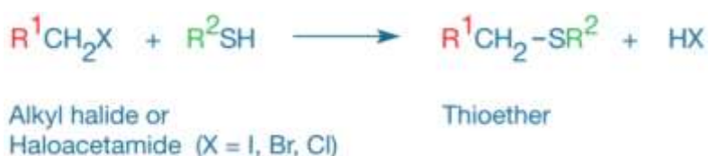
Figure 9. Reaction scheme of a thiol with an alkyl halide. 43
