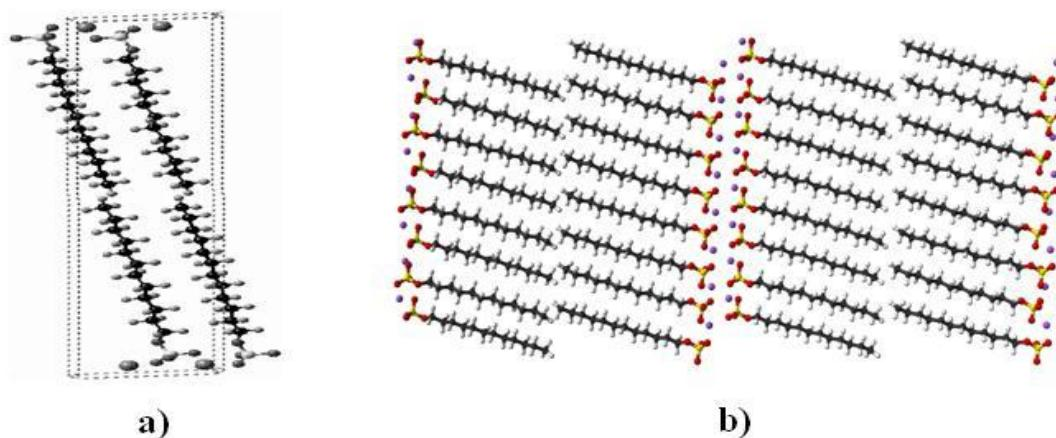
**Slika 135. a)** Pakiranje molekula NaDS u monokristalu. Parametri jedinične ćelije:  $a = 38,915 \text{ \AA}$ ,  $b = 4,709 \text{ \AA}$ ,  $c = 8,198 \text{ \AA}$ ,  $\alpha = 90,00^\circ$ ,  $\beta = 93,29^\circ$ ,  $\gamma = 90,00^\circ$ ,  $V = 1499,80 \text{ \AA}^3$ .<sup>331,332</sup>
