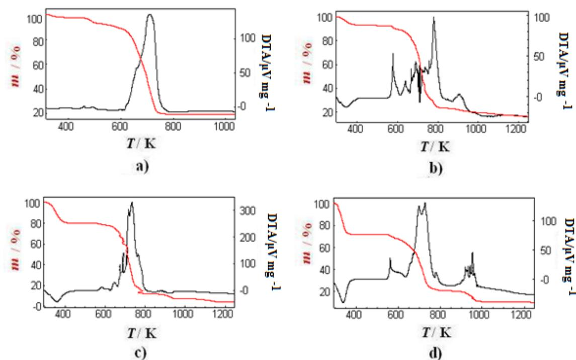
**Slika 107.** Termogrami (crvena linija) i rezultat DTA analize (crna linija) za gelove metaloamfifila: **a)** Ag–Ch<sup>G</sup>; **b)** Ba–Ch<sup>G</sup>; **c)** Ca–Ch<sup>G</sup>; **d)** La–Ch<sup>G</sup>.
