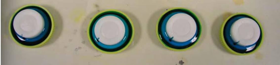
Figure 2.14. Pseudo DGT deployed in dye solution (Wagner, 2004).
