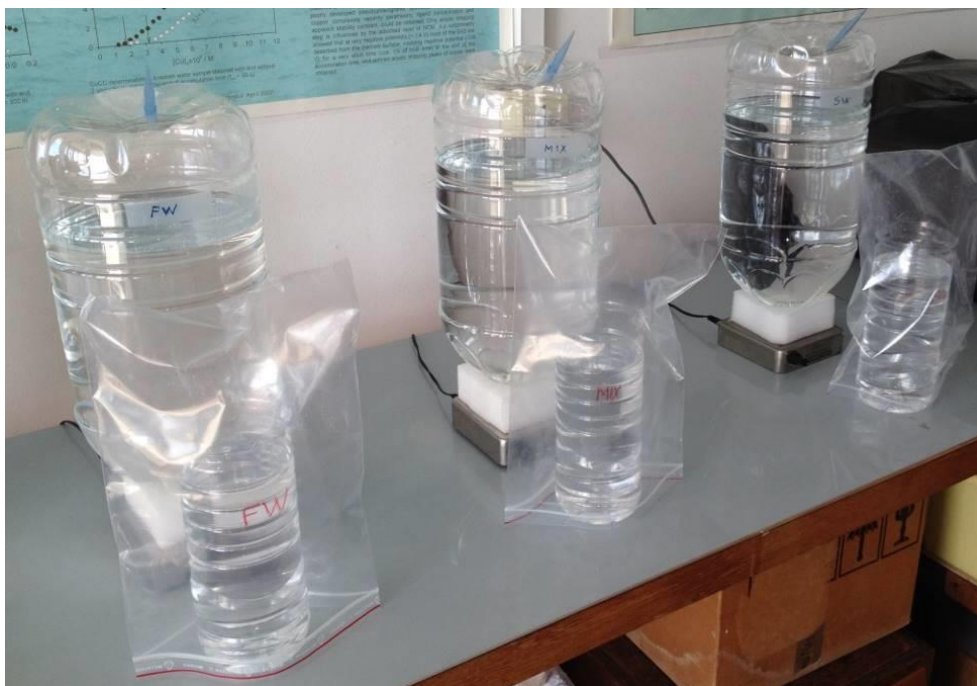
Figure 3.15. Preparation of sample for DGT diffusive coefficient determination
