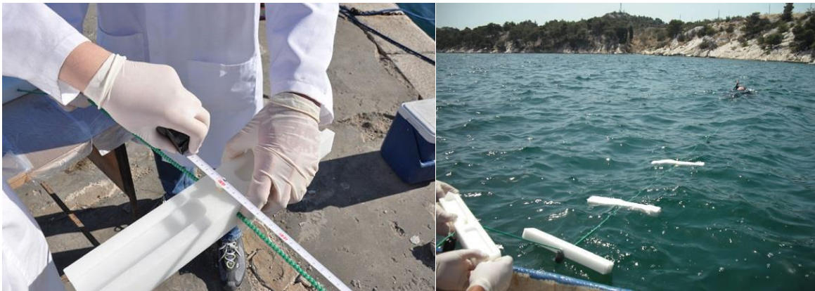
Figure 3.8. Setup of DGT holder positions (depth) and procedure of DGT deployment.
