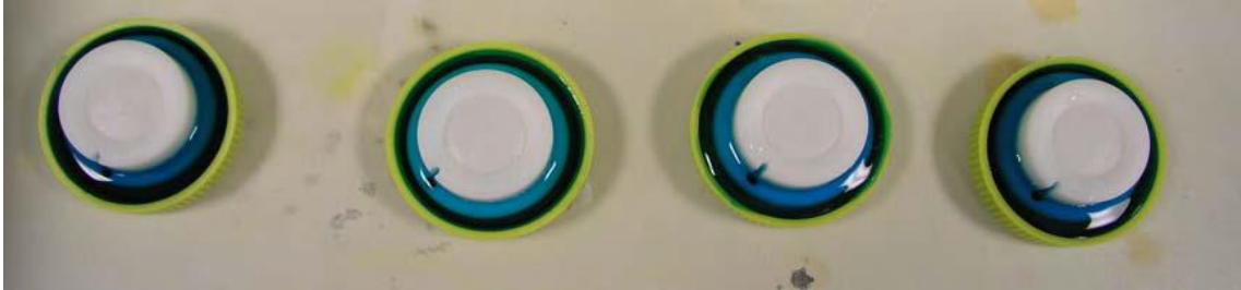
Figure 2.14. Pseudo DGT deployed in dye solution (Wagner, 2004).
