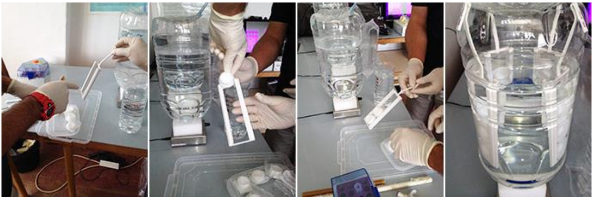
Figure 3.16. Set up for DGT “diffusion coefficient” experiment
