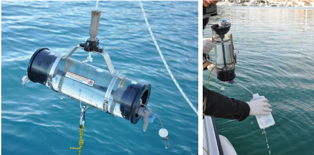
Figure 3.4. Horizontal water sampler, and the filling of a FEP bottle with a sample taken with the horizontal sampler
