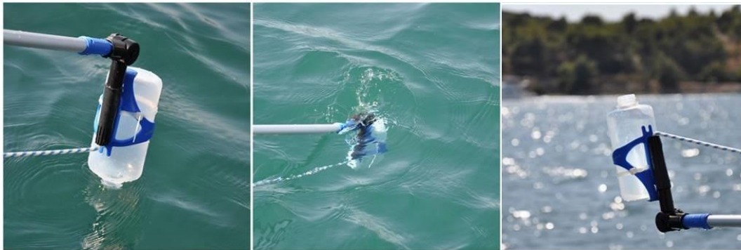
Figure 3.5. Grab sampling of the surface layer during “cross-section” and „high-resolution“ sampling.
