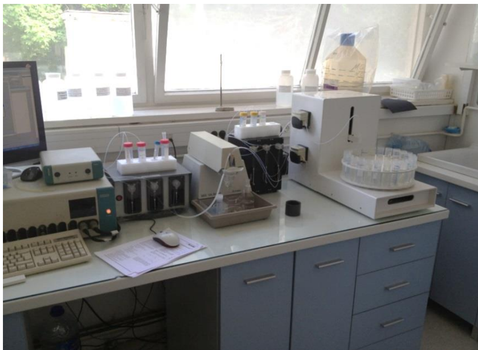
Figure 3.14. Automated voltammetric system for trace metals analysis
