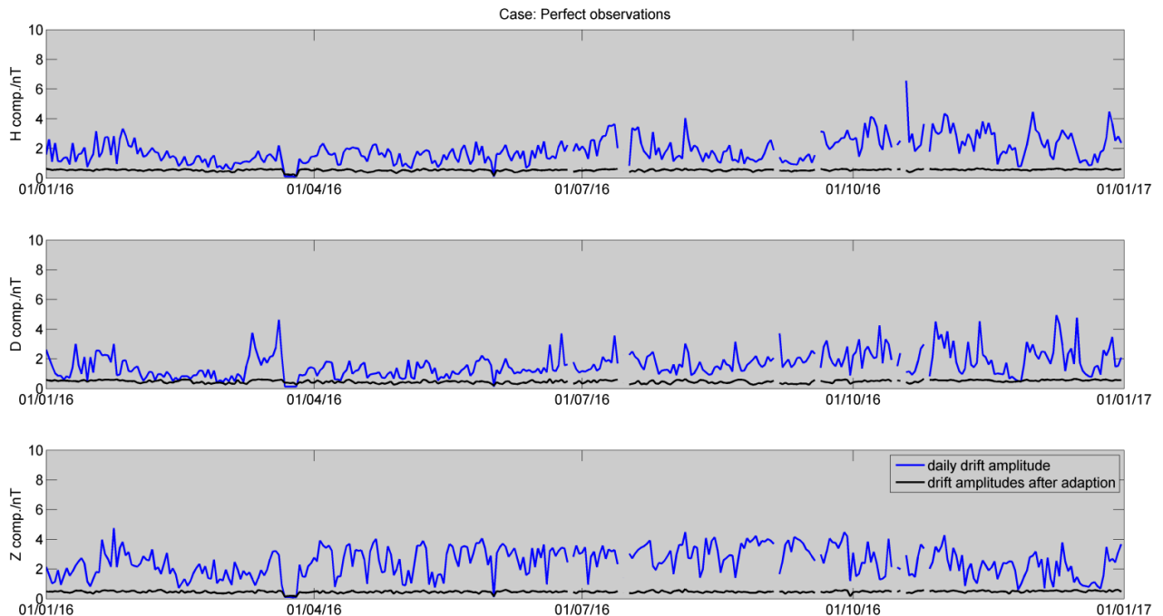
Figure 5.7 Daily drift amplitudes of uncorrected LEMI series (blue line). Drift amplitudes after calibration of LEMI series with “perfect” observations (black line).
