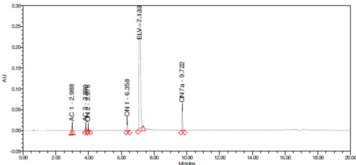
Slika D43. Kromatogram otopine IMP 2.1 pri uvjetima  $t = 15 \text{ min}$ ,  $T = 60 \text{ }^{\circ}\text{C}$  i  $\text{pH} = 8,9$
