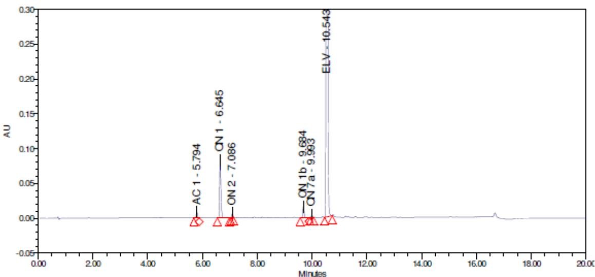
Slika D44. Kromatogram otopine IMP 2.2 pri uvjetima  $t = 15 \text{ min}$ ,  $T = 60 \text{ }^{\circ}\text{C}$  i  $\text{pH} = 8,9$
