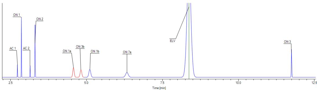
**Slika 19.** DryLab kromatogram pri uvjetima  $t = 15 \text{ min}$ ,  $T = 60^\circ\text{C}$ ,  $\text{pH} = 2,1$  i protok  $0,8 \text{ mL min}^{-1}$
