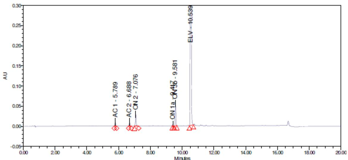
Slika D18. Kromatogram otopine IMP 1.2 pri uvjetima  $t = 15 \text{ min}$ ,  $T = 30 \text{ }^{\circ}\text{C}$  i  $\text{pH} = 6,8$
