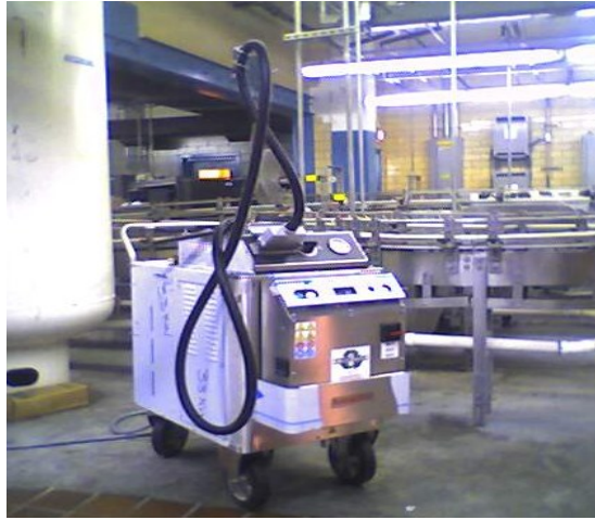
Slika 4. Oprema za fizikalno uklanjanje biofilma u prehrambenoj industriji ( http://www.cleaning-with-steam.com/remove-and-kill-biofilms-in-food-plants.html )
