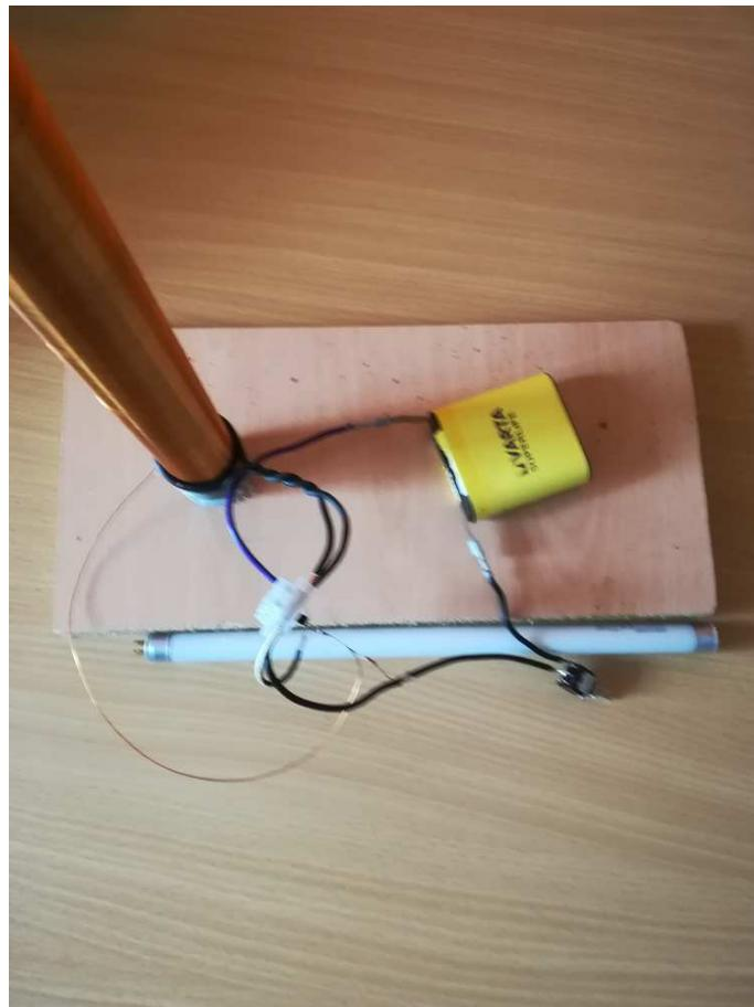
Slika 5.17: Teslin transformator
