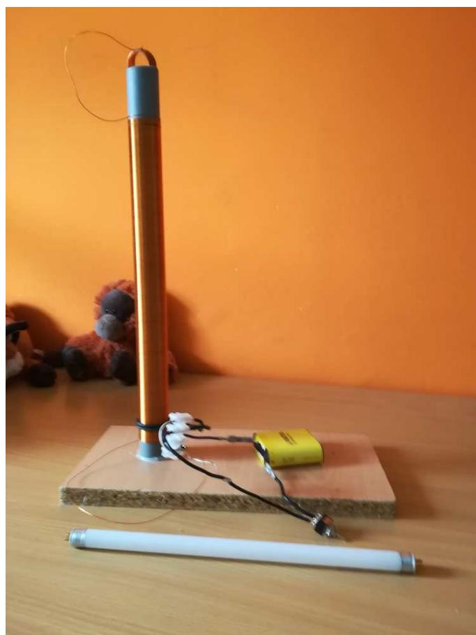
Slika 5.16: Teslin transformator
