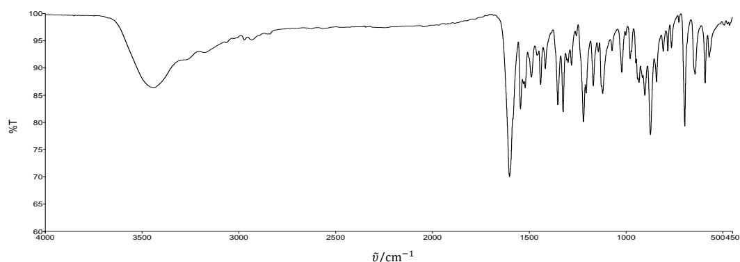
Dodatak 11. Infracrveni spektar  $[\text{MoO}_2(\text{VanHB})(\text{OH}_2)] \cdot \text{H}_2\text{O}$ , produkta reakcije  $[\text{MoO}_2(\text{acac})_2]$  i  $\text{H}_2\text{VanHB}$  u acetonitrilu
