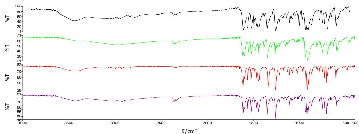
Dodatak 27. Usporedba infracrvenog spektra  $[\text{MoO}_2(\text{VanHB})]_n \cdot n\text{CH}_3\text{CN}$  (crno) sa spektrima produkata otapanja  $[\text{MoO}_2(\text{SalHB})(\text{MeOH})]$  (zeleno) i  $[\text{MoO}_2(4-\text{OMeSalHB})(\text{MeOH})]$  (plavo) u acetonitrilu
