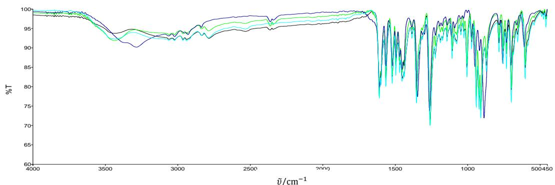
Dodatak 9. Infracrveni spektar  $[\text{MoO}_2(\text{SalHB})(\text{OH}_2)] \cdot \text{H}_2\text{O}$ , produkta reakcije  $[\text{MoO}_2(\text{acac})_2]$  i  $\text{H}_2\text{SalHB}$  u acetonitrilu
