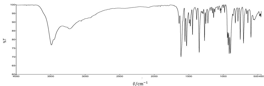
Dodatak 10. Infracrveni spektar  $[\text{MoO}_2(4-\text{OMeSalHB})(\text{OH}_2)]$ , produkta reakcije  $[\text{MoO}_2(\text{acac})_2]$  i  $\text{H}_24-\text{OMeSalHB}$  u acetonitrilu
