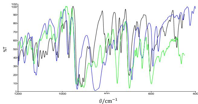
Slika 31. Usporedba infracrvenog spektra  $[\text{MoO}_2(\text{VanHB})]_n \cdot n\text{CH}_3\text{CN}$  (crno) sa spektrima produkata otapanja  $[\text{MoO}_2(\text{SalHB})(\text{MeOH})]$  (zeleno) i  $[\text{MoO}_2(4-\text{OMeSalHB})(\text{MeOH})]$  (plavo) u acetonitrilu u području valnih brojeva  $1200\text{ cm}^{-1} - 400\text{ cm}^{-1}$
