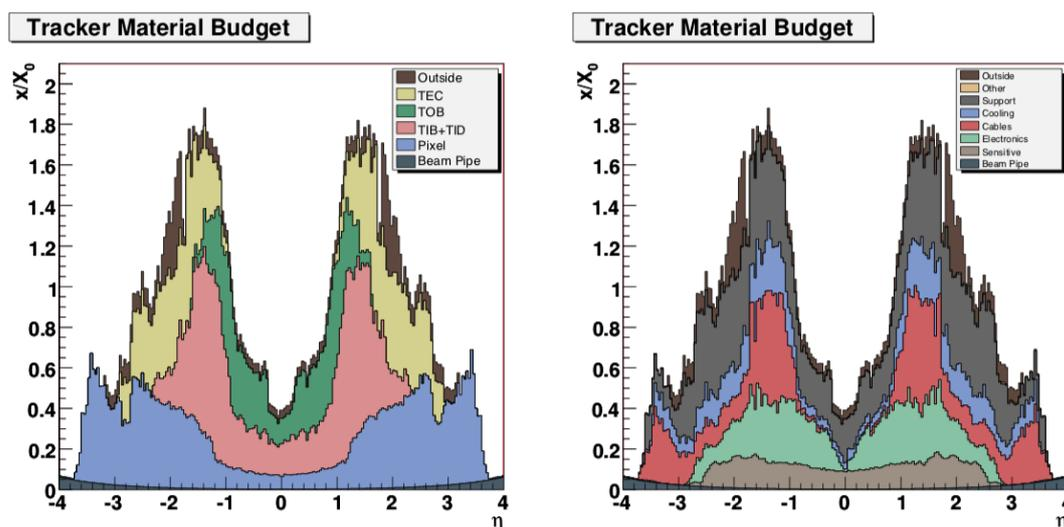
Figure 4.4: Material budget in units of radiation length as a function of pseudorapidity  $\eta$ , for the different sub-detectors (left panel) and broken down into the functional contributions (right panel).
