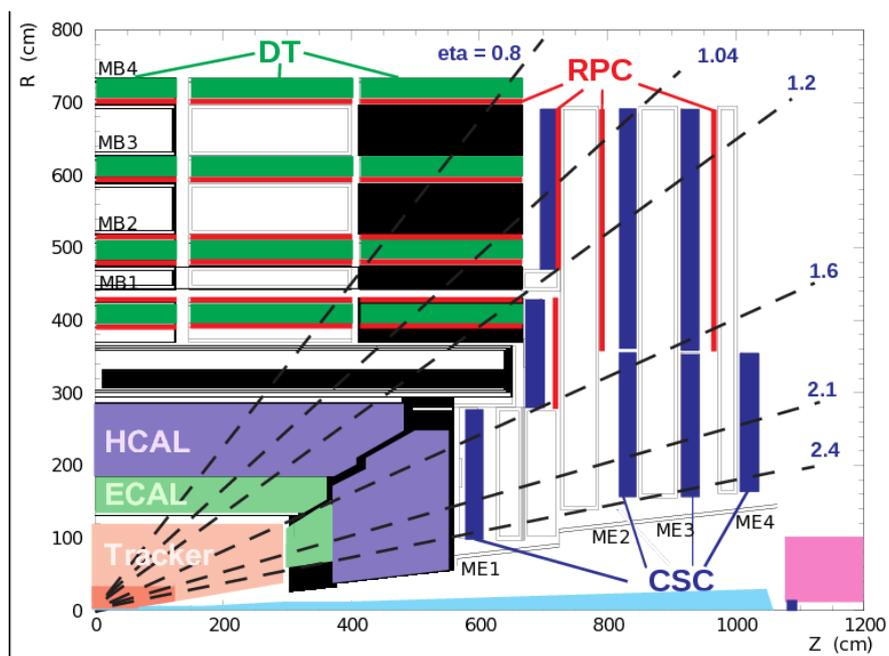
Figure 4.10: Geometric view of the CMS muon system, demonstrating the  $\eta$  barrel (MB1–MB4, green), the four CSC stations in the endcap (ME1–ME4, blue), and the RPC coverage and overlap of all constituent subsystems.
