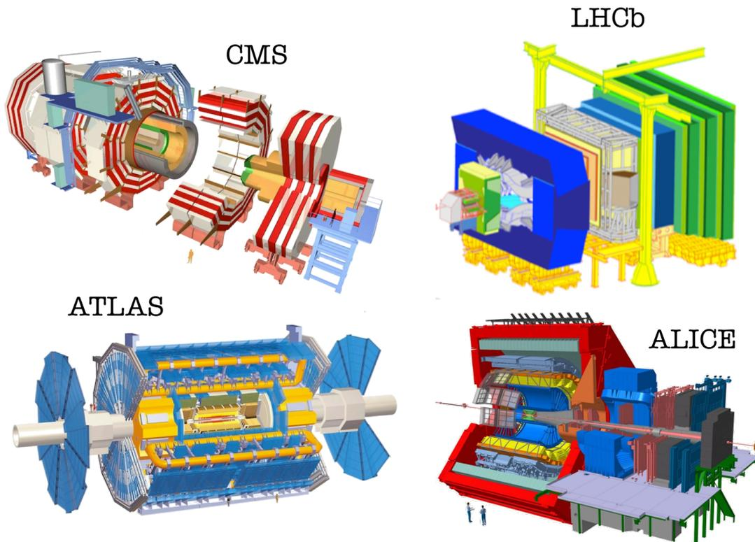
Figure 3.5: Schematic perspective view of the four main experiments installed at the LHC. From the top left, clockwise: CMS, LHCb, ATLAS and ALICE.
