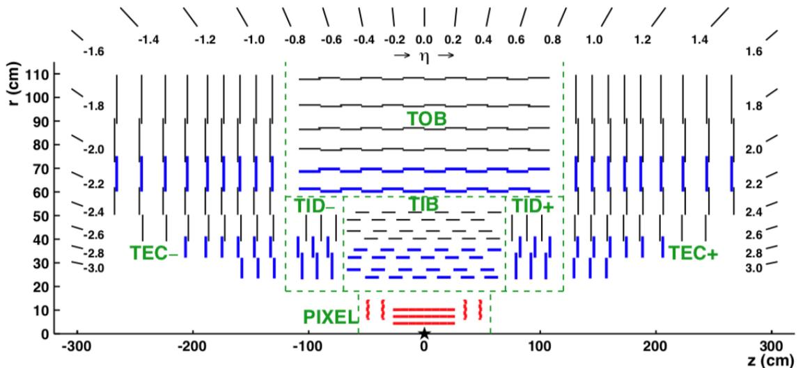
Figure 4.6: Schematic cross section through the CMS tracker in the  $r$ - $z$  plane. In this view, the tracker is symmetric about the horizontal line  $r = 0$ , so only the top half is shown here. The centre of the tracker, corresponding to the approximate position of the  $pp$  collision point, is indicated by a star. Green dashed lines help the reader understand which modules belong to each of the named tracker subsystems.
