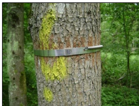
Figure 2.6: Tree with installed dendrometer band
