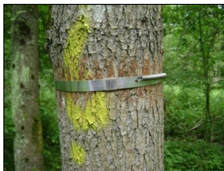
Figure 2.6: Tree with installed dendrometer band
