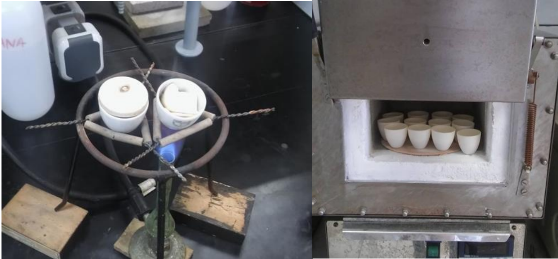
Figure 13. A – smoking the filter paper with precipitated BaSO 4 over a gas burner; B – porcelain crucibles with precipitated BaSO 4 in cold muffle furnace.
