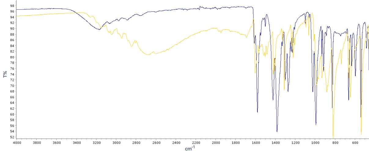
**D14.** IR spektar  $[\text{Ni}(\text{Cl-acac})_2(4\text{-oxy})_2]$  (tamnoplavo) i liganda 4-oxy (žuto).
