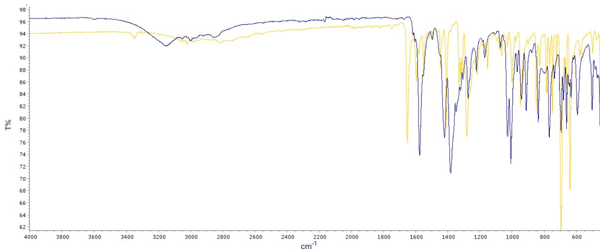
**D20.** IR spektar  $[\text{Ni}(\text{Cl-acac})_2(4\text{-phoxy})_2]$  (tamnoplavo) i liganda 4-phoxy (žuto).
