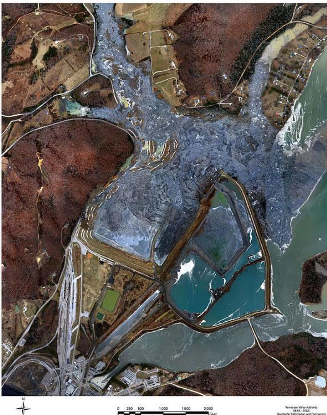
Sl. 6. Prikaz onečišćenog područja otpadnih voda iz termoelektrane na ugljen TVA *Kingston Fossil Plant*. Izvor: [http://www.wikiwand.com/en/Kingston\\_Fossil\\_Plant\\_coal\\_fly\\_ash\\_slurry\\_spill](http://www.wikiwand.com/en/Kingston_Fossil_Plant_coal_fly_ash_slurry_spill)
