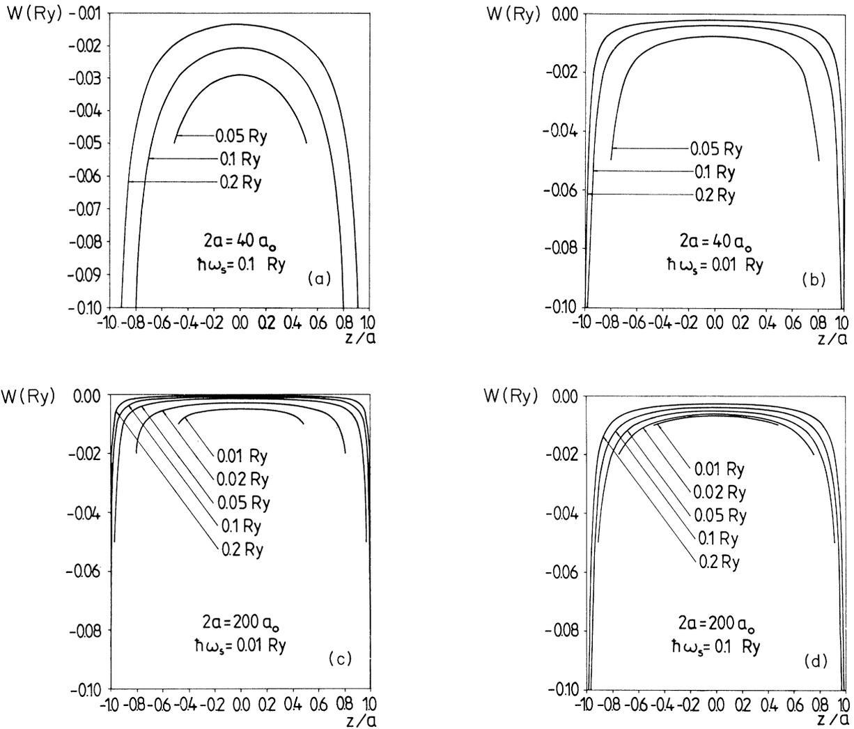
FIG. 1. Self-consistently calculated dynamical image potentials in the barriers of widths  $2a = 40a_0$  and  $200a_0$ , in the first iteration. The SP energies are  $\hbar\omega_s = 0.1$  and  $0.01$  Ry,  $m^* = 0.07m$ . The electron energies are 0.01, 0.02, 0.05, 0.1, and 0.2 Ry.
