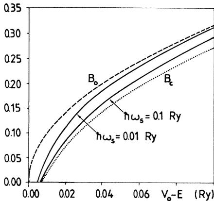
FIG. 2. Tunneling rates for the barrier with  $2a = 200a_0$ ,  $m^* = 0.07m$ , calculated with no image potential ( $B_0$ ), classical image potential ( $B_c$ ), and the dynamical image potential ( $B$ ) for two SP frequencies:  $\hbar\omega_s = 0.1$  and  $0.01$  Ry. The rates are given in units of  $(2a/a_0)(m^*/m)^{1/2}$ .
