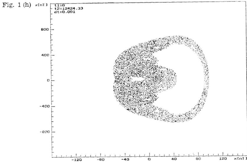
Fig. 1. Poincaré maps for robotic equation (1) with parametrization (I) and the characteristic values of the control parameter  $L$ : (a)  $L = 0.1$ , (b)  $L = 1$ , (c)  $L = 37$ , (d)  $L = 47$ , (e)  $L = 48$ , (f)  $L = 49$ , (g)  $L = 74$ , (h)  $L = 99$ .
