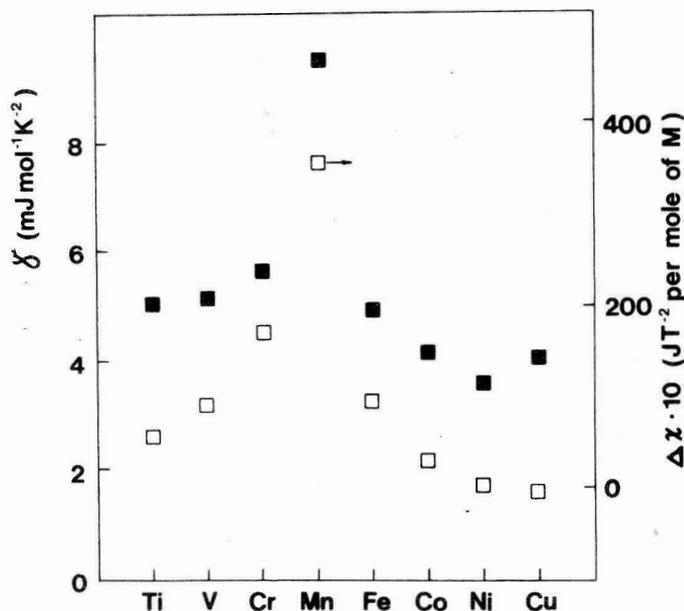
Fig. 2. Electronic specific heat coefficient  $\gamma$  for amorphous  $(\text{Ni}_{33}\text{Zr}_{67})_{85}\text{M}_{15}$  alloys (■) and the change in magnetic susceptibility  $\Delta\chi$  (□) per mole of M of amorphous  $\text{Zr}_2(\text{Ni}_{1-x}\text{M}_x)_1$  alloys vs M.
