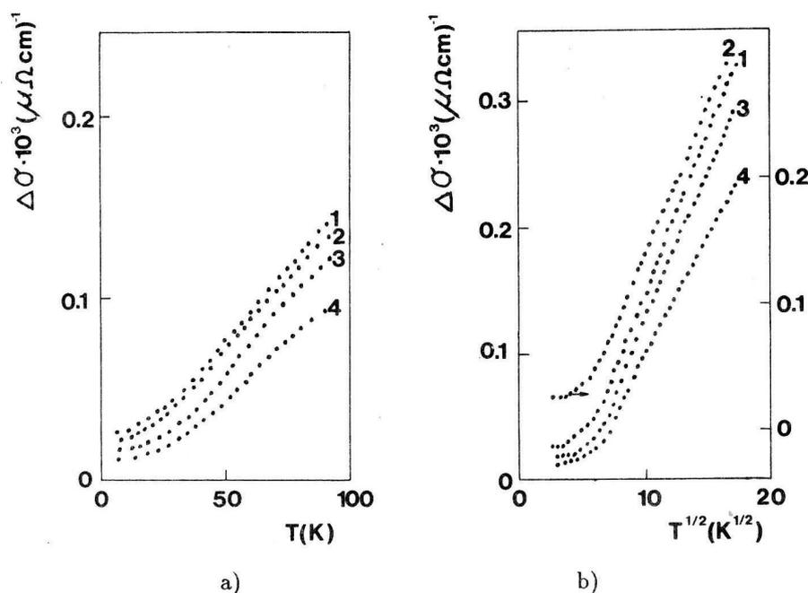
Fig. 1. Change in electric conductivity  $\Delta\sigma = \sigma_T - \sigma_0$  for selected  $\text{Zr}_2(\text{Ni}_{1-x}\text{M}_x)_1$  glassy alloys vs.  $T$  (a) and  $T^{1/2}$  (b): (1)  $\text{Zr}_2(\text{Ni}_{0.9}\text{Co}_{0.1})_1$ , (2)  $\text{Zr}_2(\text{Ni}_{0.8}\text{Ti}_{0.2})_1$ , (3)  $\text{Zr}_2(\text{Ni}_{0.5}\text{Fe}_{0.5})_1$  and (4)  $\text{Zr}_2(\text{Ni}_{0.9}\text{Mn}_{0.1})_1$ .
