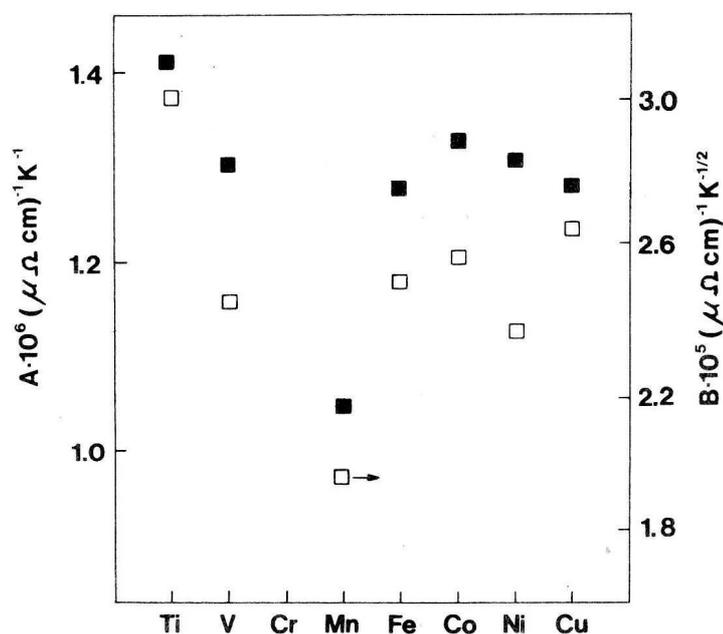
Fig. 3. Coefficient  $A$  of linear conductivity variation below 100 K (■) and coefficient  $B$  of a  $T^{1/2}$  conductivity variation (□) above 100 K vs M.
