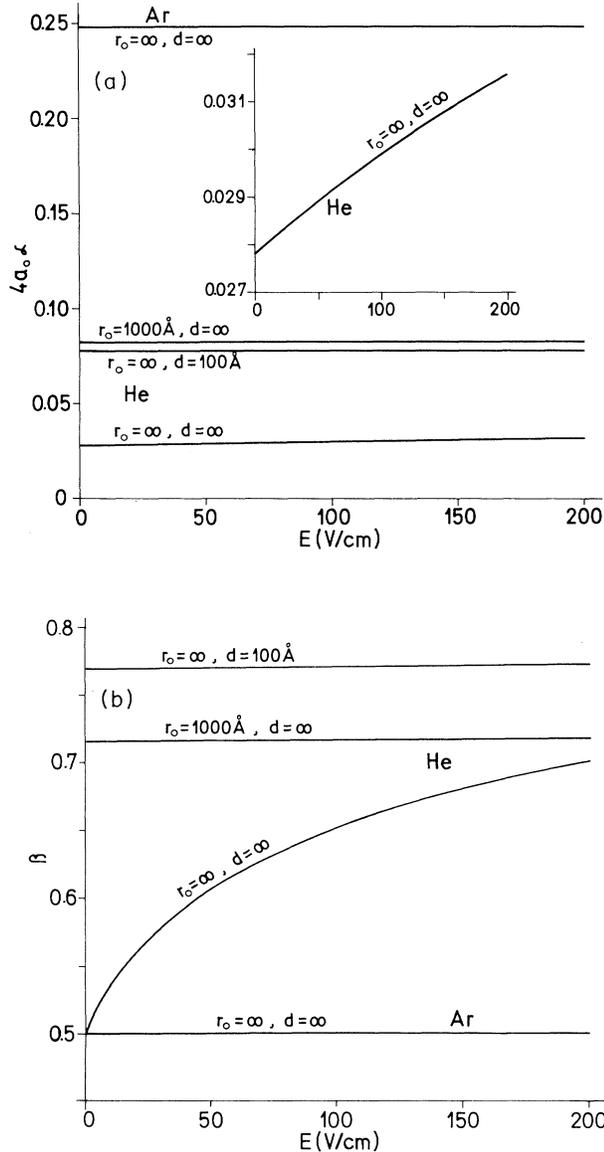
FIG. 3. Optimized values of (a)  $\alpha$  [in units  $(4a_0)^{-1}$ ,  $a_0$  is the Bohr radius] and (b)  $\beta$  for the Wigner lattice as functions of external electric field  $E$ . The inset of (a) shows the small change of  $\alpha$  even in the case of the He substrate in the  $(r_0 \rightarrow \infty, d \rightarrow \infty)$  limit. The Ar substrate gives in all cases almost constant values of both parameters  $(\alpha, \beta)$ .
