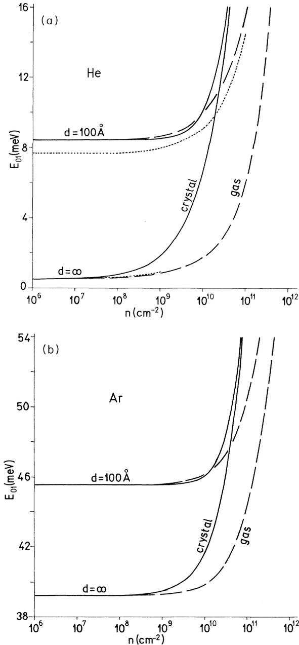
FIG. 2. Excitation energies  $E_{01} = E_1 - E_0$  of 2D electrons in the case of a crystal (full lines) and a gas (dashed lines) phase, as functions of electron density  $n$ . Two different thicknesses of (a) He and (b) Ar substrates are chosen. The dotted lines in (a)
