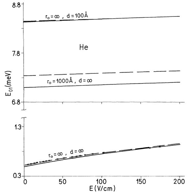
FIG. 4. Excitation energies  $E_{01}$  of the 2D Wigner lattice on the He layer, as functions of external electric field  $E$ . The correction due to electron penetration into the He surface is shown by dashed lines. The experimental values (Ref. 3) are shown by crosses.
