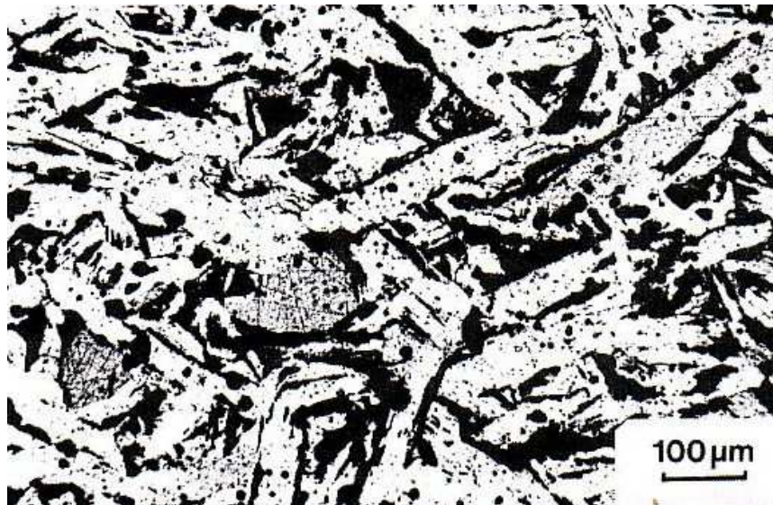
Fig. 3. Optical micrograph of the \text{YBa}_2\text{Cu}_3\text{O}_{7-x} ceramic, sample NOZ 1-III (aged for 700 hours at 960^\circ\text{C} ), polished with diamond paste and etched for 5 seconds in a mild solution of HCl in distilled water.
