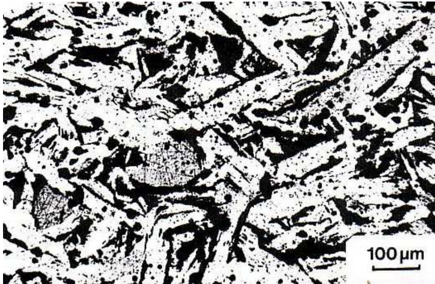
Fig. 3. Optical micrograph of the \text{YBa}_2\text{Cu}_3\text{O}_{7-x} ceramic, sample NOZ 1-III (aged for 700 hours at 960^\circ\text{C} ), polished with diamond paste and etched for 5 seconds in a mild solution of \text{HCl} in distilled water.
