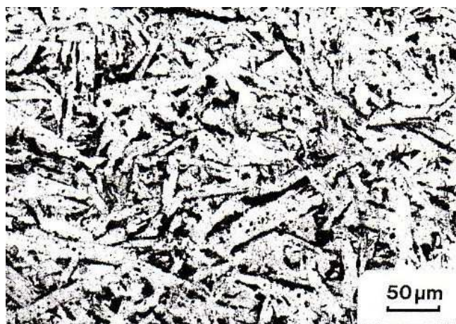
Fig. 5. Optical micrograph of NOZ 1-III, etching time 10 seconds.
