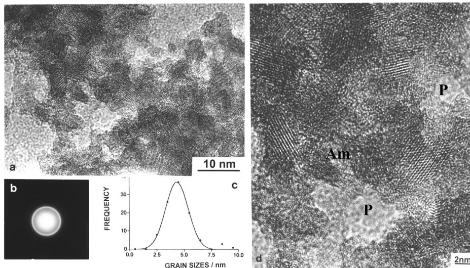
*Fig. 1.  $TiO_2$  sample S2 (starting thin solid film heated up to (573 K): a) HREM image showing nanocrystalline grains of anatase and brookite, of size  $(5 \pm 2)$  nm, and pores of size from 1.5 to 10 nm; b) the corresponding ED pattern; c) the distribution of size of grains, measured by HREM, and fitted by the Gaussian curve; d) magnified part of HREM image a); the overlapped grains, pores (P) and regions of amorphous phase (Am).*
