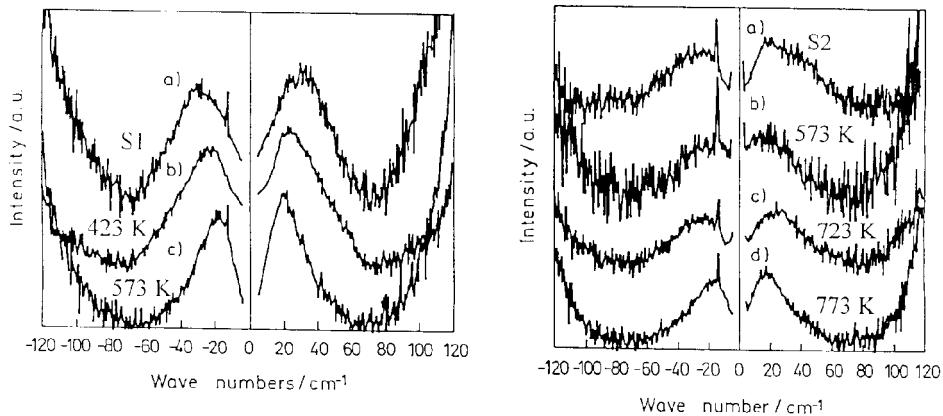
Fig. 5. Low-frequency Raman modes at about  $20\text{ cm}^{-1}$  after baseline and temperature corrections. a)  $\text{TiO}_2$  sample S1 (starting sample) and samples heated to 423 and 573 K; b)  $\text{TiO}_2$  sample S2 (starting sample) and samples heated to 573, 723 and 773 K.
