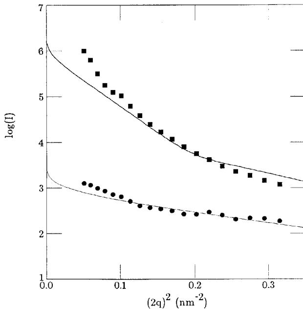
Fig. 4. SAXS data for the sample S2, not-heated (squares) and heated to 773 K (circles): Guinier plot relating  $\log I$  and  $(2q)^2$ , where  $I$  is the scattered intensity, and  $q$  the wave vector in  $\text{nm}^{-1}$ .
