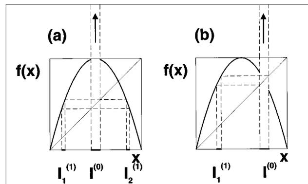
FIG. 1. Logistic map at  $r=4$  with an additional hole of width  $d$  at the position  $\xi$  on the unit interval [Eq. (1)]. As an illustration, the hole position is (a)  $\xi=0.5$ , (b)  $\xi=0.75$ , and the hole width is  $d=0.1$ . Only the first order preimages are shown. Observe that the preimage  $I_2^{(1)}$  is missing for  $\xi=0.75$ .
