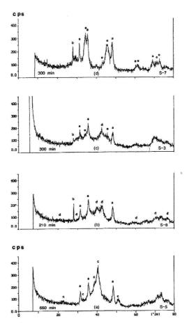
Fig. 3. XRD patterns taken from various powder mixtures milled in air atmosphere and at room temperature: (a) S-5 (W:B=2:1), (b) S-6 (W:B=1:1), (c) S-3 (W:B=2:5) and (d) S-7 (W:B=1:4). The numbers denote milling times; the angular positions of the observed diffraction lines belonging to the tungsten boride crystalline phases are marked as follows: (c)  $W_2B$ , (d) WB and (e)  $WB_4$ , while for those phases mentioned in Fig. 2 the same simbols are used.
