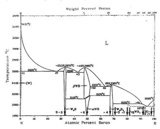
Fig. 1. The equilibrium W-B phase diagram [5]. The arrows denote the compositions of elemental powder mixtures studied in the present work.
